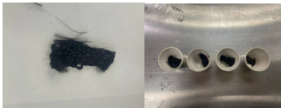
Figure 3. Samples after pyrolysis under 600 °C.
