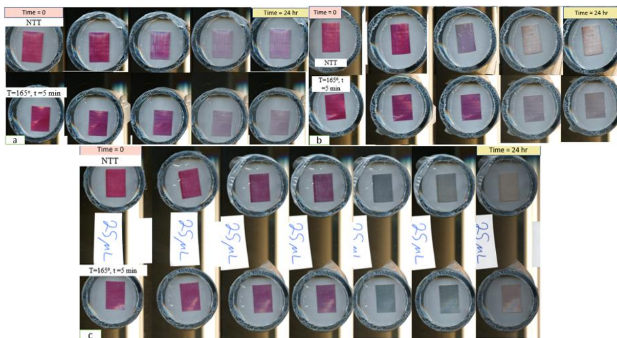
Figure 4.7 Sensitivity test for examining the response of pH indicator towards TMA, a = 25 \mu L, b = 10 \mu L, c = 5 \mu L of trimethylamine solution.
