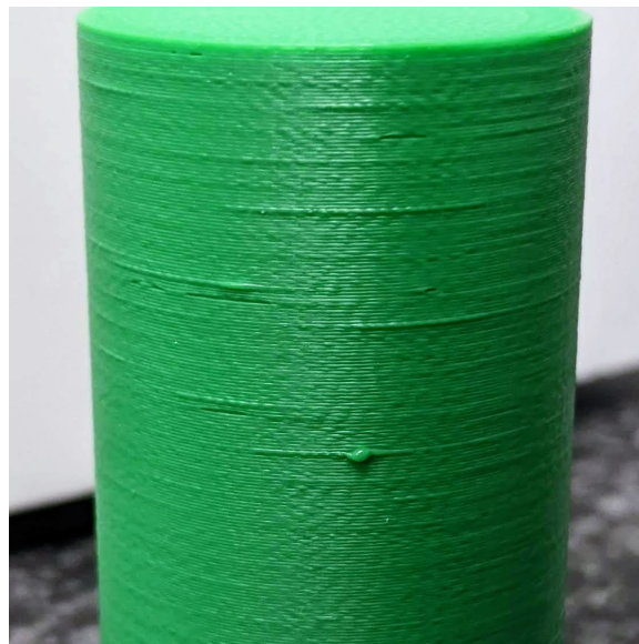
Figure 1. Random errors on the surface of a cylindrical 3D printed part occurring on a single layer. They often present themselves as horizontal streaks or bumps on the surface of the printed part.
