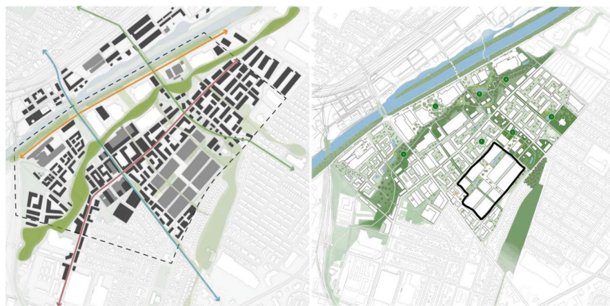
Fig. 2.5 Master plan. The revitalization project for the North Lasalle area, south of the Lachine Canal, proposed by a team of 5 students. On the left, the proposed new densification (black buildings) and building renovation strategy (dark gray buildings). On the right, the proposed biodiversity and greening strategy. Note the green corridor strategy that runs along an existing embankment parallel to the Lachine Canal. The Montreal CIL complex is identified in black on the right-side map (the site analyzed in Sect. 3). (Source: Marylou Filiatrault, Janie Ouellette, Charlie Proteau, Alexandra Thibodeau-Gagnon, Godefroy Vallette)
