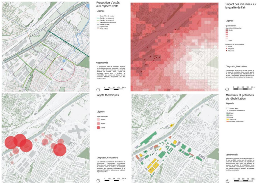
Fig. 2.4 Urban Diagnosis based on the Urban Ecology Agency of Barcelona’s Ecological Urbanism framework for the Dominion/North Lasalle North zone, with indicators for access to green spaces, impact of industries on air quality, thermal waste, and rehabilitation potential. (Source: Janie Ouellette, Olivier Pesant and Jordane Castonguay, 2022)
