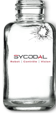
Figure 4.4 Glass Bottle: Open Mark Defect
