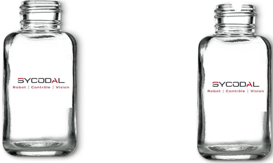
Figure 4.2 Defective vs Non-Defective Glass Bottle
