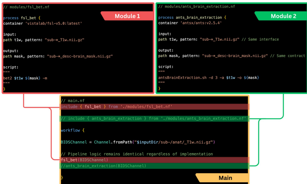
Fig. 3 Example Nextflow snippets demonstrating how different processes—FSL (red, fsl_bet.nf ) and ANTs (green, ants_brain_extraction.nf )—performing equivalent tasks through standardized input/output
