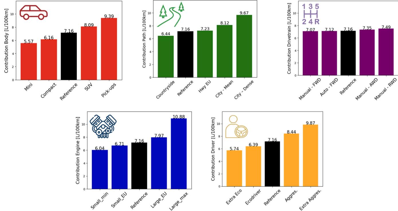
**Figure 5.** Computation of energy consumption for twenty-one GV pre-set configurations. The average European GV is shown as the reference. Alternative scenarios, which vary one contributor at a time, are classified by the contributor affected: the body (red), the engine (blue), the path (green), the driver (yellow), and the drivetrain (purple). (For interpretation of the references to color in this figure legend, the reader is referred to the Web version of this article.)
