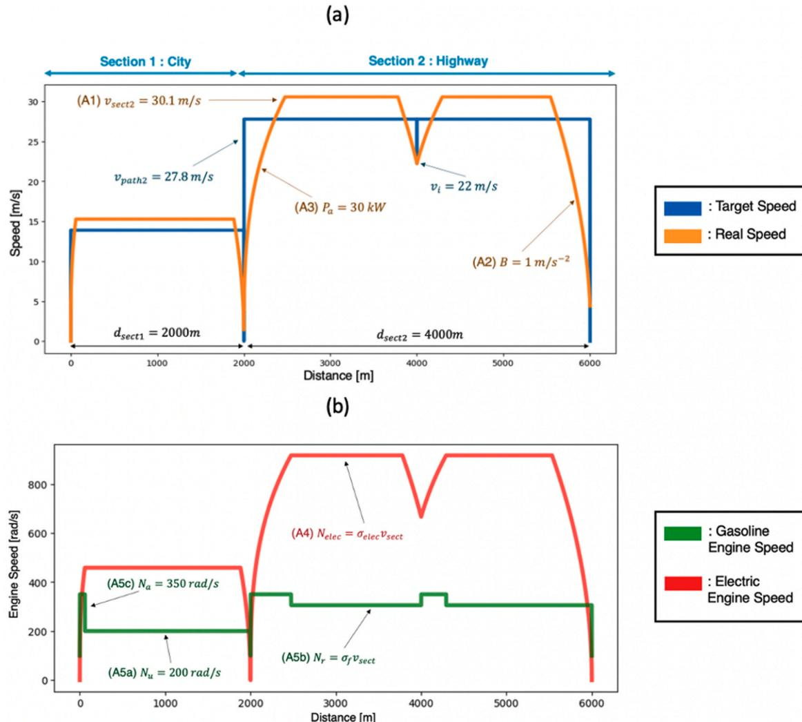
**Figure 2.** Graphical Representation of the Integration Method for a theoretical travel of 6 km with 2 km of urban travel and 4 km of highway travel. a) represents the target speed (in blue) and the real speed (in orange) functions, and b) represents the real engine speed functions for ICEV and BEV. (For interpretation of the references to color in this figure legend, the reader is referred to the Web version of this article.)
