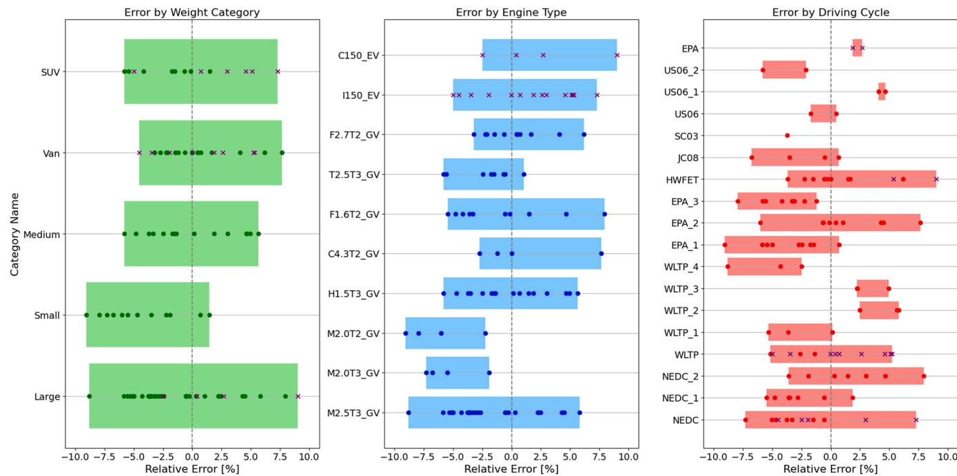
**Figure 4.** Distribution of the relative error between parametrized model and manufacturer empirical energy consumption measurements. Each point (for GV) and cross (for BEV) represents a single simulation. Shaded regions indicate the range of relative errors for each category. Simulations are classified by:
