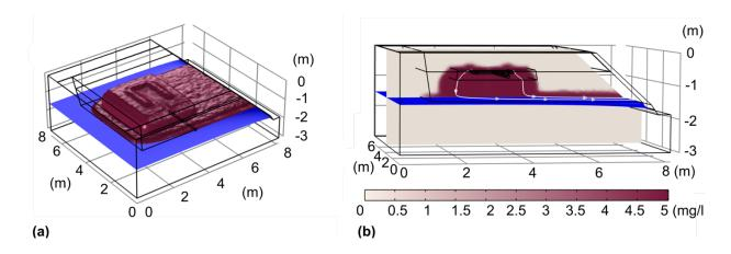
Figure S5- Model 1 3D simulation in day 360. (a) Isosurface of 4 mg/l of P and water table and (b) water table, contour map of P concentration and streamlines in a cross-section.
