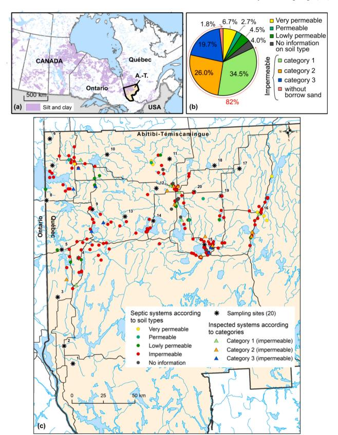
Fig. 1. (a) Map of Abitibi-Témiscamingue in Québec, Canada and silt and clay coverings [54-56]. (b) Classification of documented systems based on soil type and system category, (c) Location of documented systems with their settings' permeability, sampling sites and inspected systems.
