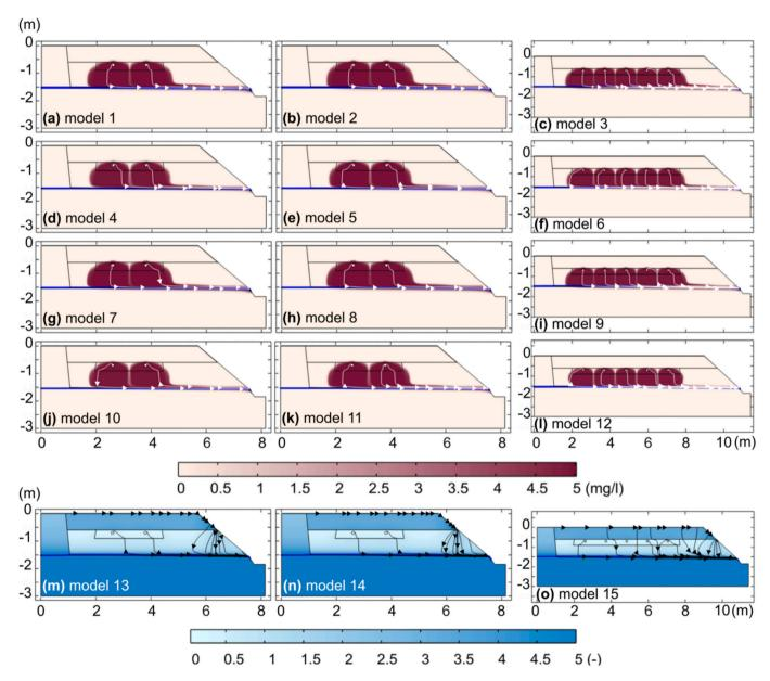
Fig. 6. 2D contour maps of P concentration, water table (blue line), and streamlines, (a–f) models 1–6 in day 360, (g–l) models 7–12 in day 180. 2D contours of saturation degree and streamlines, (m–o) models 12–15 after 24 h of heavy rain. (For interpretation of the references to colour in this figure legend, the reader is referred to the web version of this article.)
