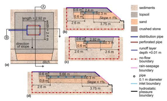
Fig. 3. Simulated polishing beds and the implemented boundary conditions. (a) Plan of a polishing bed for 1-bedroom residences. The dashed line shows the boundaries of the crushed stone layer. (b) Cross-section A simulated for polishing beds for 1-bedroom residences and rectangular polishing beds for 6-bedroom residences. (c) Cross-section B considered for 3D simulation of model 1. (d) Cross-section simulated for all square polishing beds for 6-bedroom residences.
