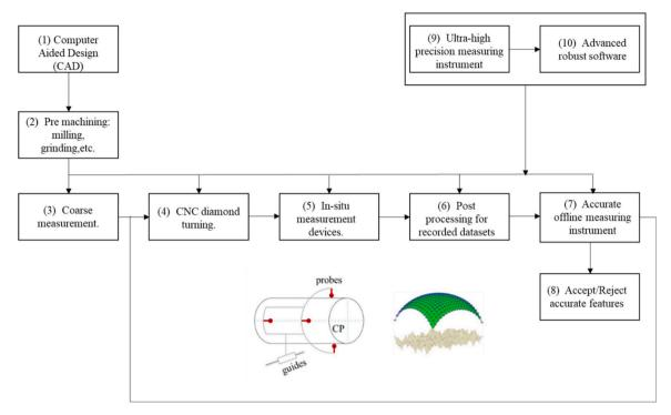
Fig. 1. Iterative process chain for ultra-accurate manufacturing.
