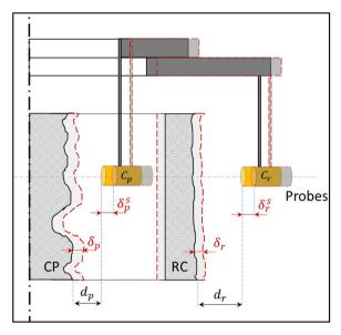
**Fig. 13.** Schematic of the symmetric configuration of the NanoCyl measuring elements (sensors and carriage structure). The expanded components are represented is red colour. RC=Reference Cylinder.
