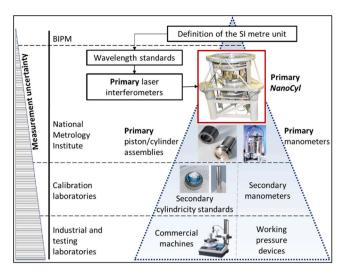
**Fig. 3.** Established traceability for cylindricity measurements for piston-cylinder assemblies and material CP transfer standards.
