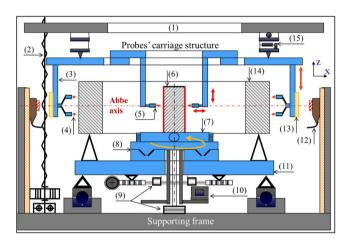
**Fig. 4.** Architecture of the primary NanoCyl applying the Precision Design Principles [15]: (1) XY translation table, (2) linear guidance, (3) metrology frame, (4) reference probes, (5) measuring probes, (6) cylindrical part, (7) automated tilt/centre table, (8) rotary indexing table, (9) encoders, (10) brake, (11) rotary table, (12) laser interferometers, (13) reflective mirror, (14) reference cylinder, (15) piezoelectric actuators.
