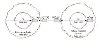
Fig. 9. Revisiting reversal error separation technique.  $M_0^{Cp}$  and  $M_{180}^{Cp}$  in the above text.
