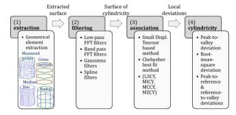
Fig. 11. Implemented strategy for evaluating the cylindricity, including the extraction and combination of the three elements (cross-section deviations, median line and radial deviations).
