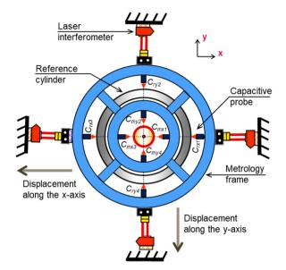
Fig. 6. Calibration of Capacitive Probes using laser interferometers [15].
