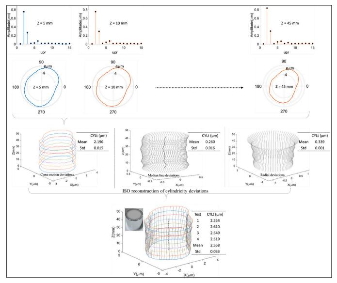
Fig. 12. Cylindricity calibration of the selected high-quality CP including the three simple elements with respect to ISO 12180.
