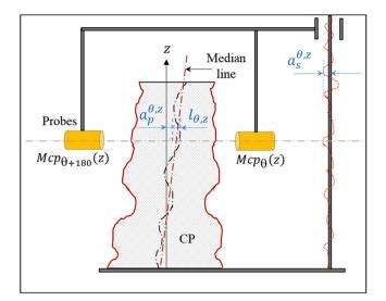
Fig. 10. Opposite probes for radial deviations detection.
