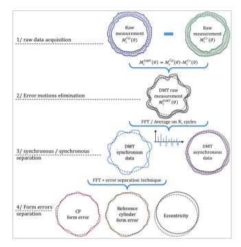
Fig. 8. Schematic diagram of the processing strategy.
