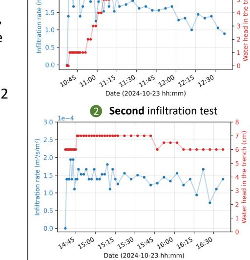
Measured data for the two successive tests
