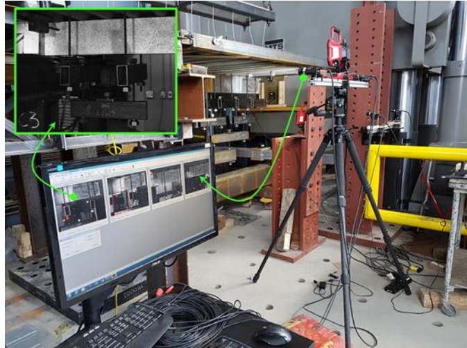
Figure 4-12: Digital image correlation system.
