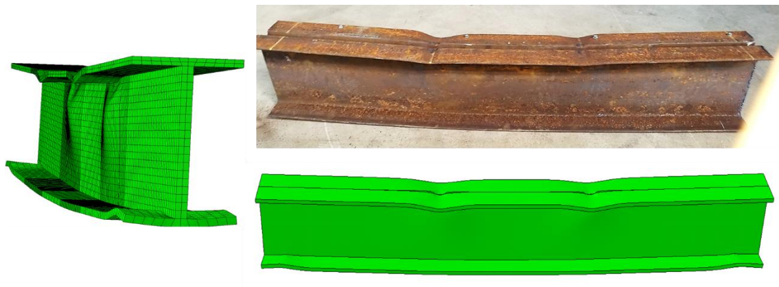
Figure 5-10: Comparison of the predicted and observed deformed shapes at the end of the bending test on the C200x17 shapes.
