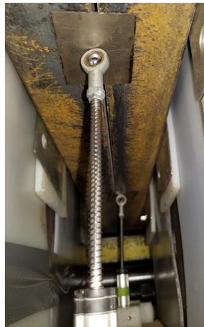
Figure 4-16: LVDT sensors used to read the vertical deflections in four-point bending tests.
