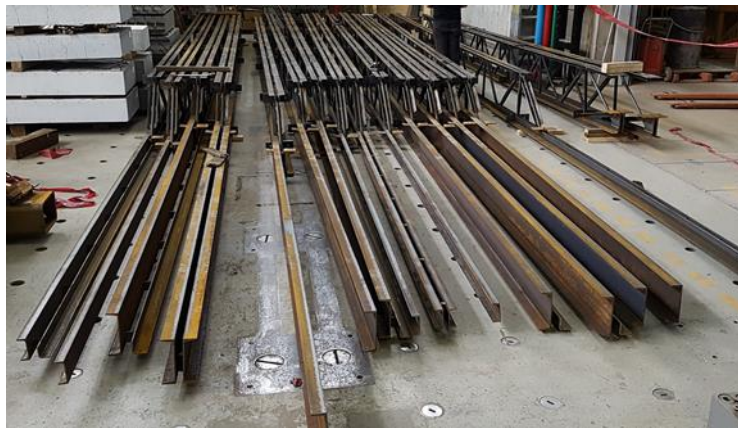
Figure 4-3: Steel joist test specimens with top chord extensions as delivered in the laboratory.
