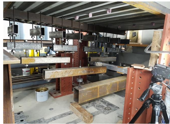
Figure 4-10: Uniformly distributed loading system.
