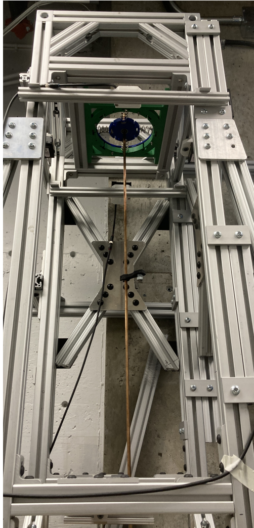
Figure 5.2 A photograph of the VARM built and tested at Polytechnique Montréal. For reference, the shaft length from the upper bearing to the lower bearing is 850 mm.
