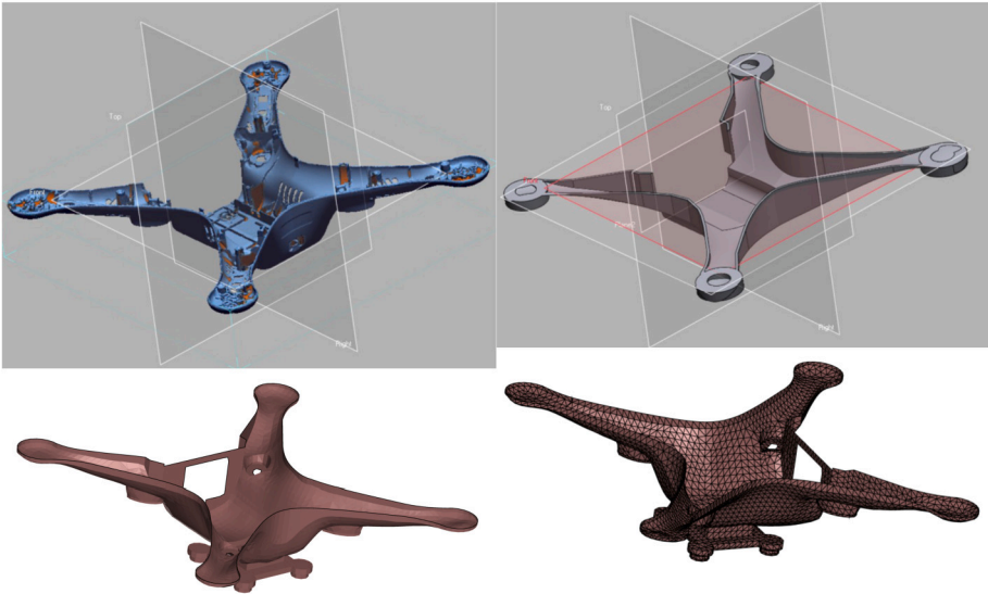
Fig. 5. Top left: cloud of points from scanned bottom casing viewed in Geomagic. Top right: de-featured casing. Bottom left: shell version of bottom casing. Bottom right: bottom casing meshed with shell elements.
