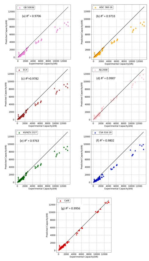
Fig. 10. Comparison between experimental and predicted axial capacity for rectangular CFSST columns by code equations and CatB model predictions.
