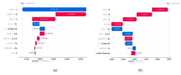
Fig. 5. Waterfall plots for (a) circular and (b) rectangular CFSST columns.
