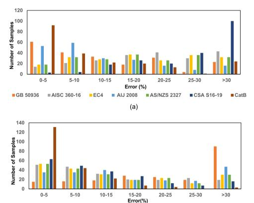
Fig. 8. Bar chart representing error ranges for (a) circular and (b) rectangular CFSST columns.
