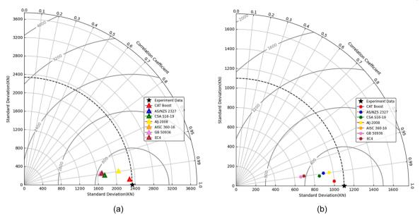
Fig. 11. Taylor Plots for (a) circular and (b) rectangular CFSST columns.
