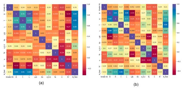
Fig. 1. Correlation matrix for (a) circular and (b) rectangular CFSST columns.
