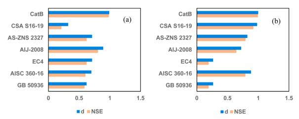
Fig. 7. Comparison between existing codes and CatB model with respect to NSE and d for (a) circular and (b) rectangular CFSST columns.
