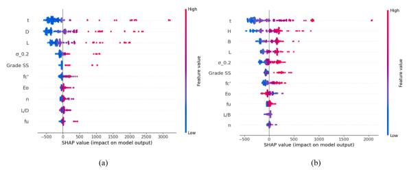
Fig. 4. SHAP summary for (a) circular and (b) rectangular CFSST columns.
