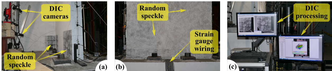
Figure 4.7 DIC instrumentation of the specimen : (a) Cameras and random speckle inside the USW ; (b) Random speckle on the exterior face of the south flange ; (c) Processing of DIC results.
