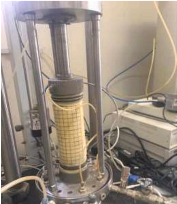
Fig. 5. Triaxial cell for freeze-thaw tests.
