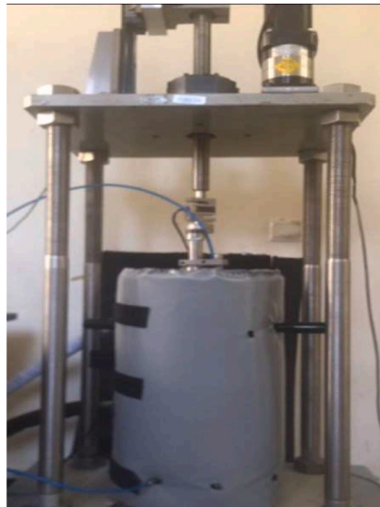
(a) External view of the cell covered by an elastomer jacket
