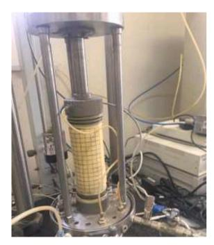
Fig. 5. Triaxial cell for freeze-thaw tests.
