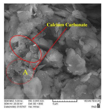
Fig. 17. Scanning Electron Microscope images of sample treated with 30 % MICP solutions and 1.5 % nano-SiO<sub>2</sub>; clear difference between clay minerals and agglomerated part.
