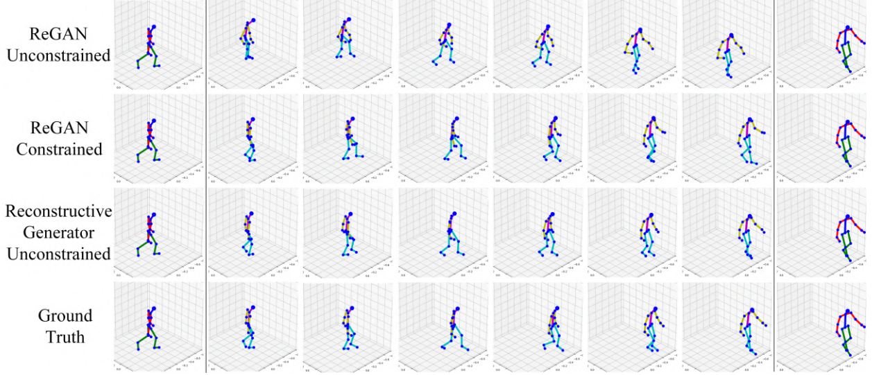
Figure 3.5 Comparison of different generated Walk-Turn transitions with the ground truth. Differences between the generated transitions are easier to observe in the supplementary video.
