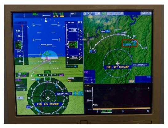
Fig. 7. Here is a picture of the display AFD-6520 Adaptive Flight Display showing the correct information for the "synthetic" aircraft with call sign "D16PSK".
