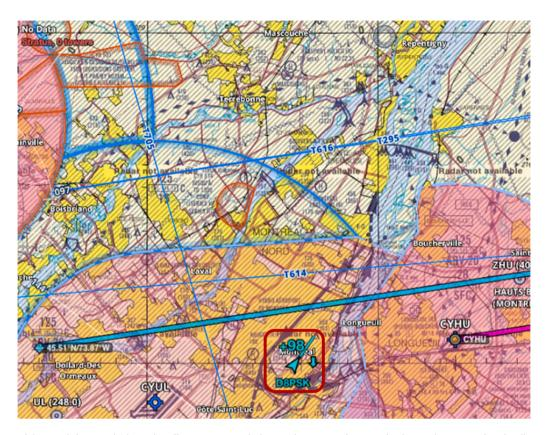
Fig. 6. Screen capture of the ForeFlight Maps display with traffic option activated, showing the correct information for the "synthetic" aircraft with call sign "D8PSK", obtained from an IPad connected to the Stratus II receiver.
