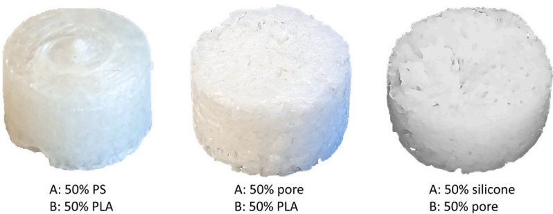
Fig. A.16. Fabrication of the silicone-based porous monoliths: PS/PLA 50/50 wt% blend is extruded, PS is selectively extracted, then silicone is injected in the PLA mold after which the PLA is also removed.
