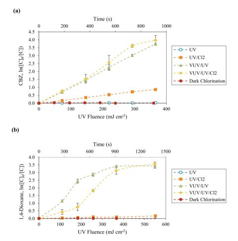
Fig. 2. Degradation of (a) CBZ and (b) 1,4-D under different AOP conditions in DI water ( $[C]_{CBZ,0} = 4 \mu M$ ,  $[C]_{1,4-D,0} = 6 \mu M$ ,  $[C]_{free\ chlorine,0} = 70 \mu M$ , Average pH = 6.5 (unadjusted)). Error bars represent the standard deviations of three experimental replicates.
