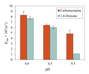
**Fig. 4.** Observed pseudo-first order rate constants for the degradation of CBZ and 1,4-D in the VUV/UV/Cl<sub>2</sub> AOP in DI water as a function of pH ([C]<sub>CBZ,0</sub> = 4  $\mu$ M, [C]<sub>1,4-D,0</sub> = 6  $\mu$ M, [C]<sub>free chlorine,0</sub> = 70  $\mu$ M, [C]<sub>phosphate buffer</sub> = 2 mM). Error bars represent the standard deviations of three experimental replicates.
