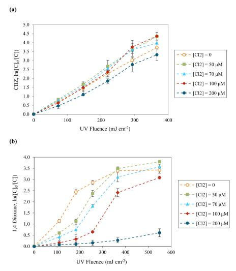
Fig. 3. Effect of free chlorine dose on the VUV/UV AOP for degradation of (a) CBZ, and (b) 1,4-D in DI water ( $[C]_{CBZ,0} = 4 \mu M$ ,  $[C]_{1,4-D,0} = 6 \mu M$ , Average pH = 6.5 (unadjusted)). Error bars represent the standard deviations of three experimental replicates.
