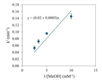
Fig. 1. (a) Experimental measurement of the pseudo-first order photo-degradation rate constant of CBZ at different concentrations of MeOH ([C]\_{CBZ,0} = 0.85 \,\mu\text{M}); (b) Estimation of the incident fluence rate at 185 nm based on the experimental results of CBZ degradation in presence of MeOH. Error bars represent the standard deviations of three experimental replicates.
