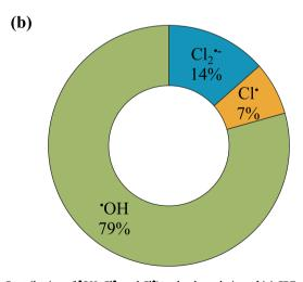
**Fig. 5.** Contribution of  ${}^{\bullet}OH$ ,  $Cl^{\bullet}$ , and  $Cl^{\bullet}$ : to the degradation of (a) CBZ and (b) 1,4-D in the VUV/UV/Cl<sub>2</sub> AOP in DI water ([C]<sub>CBZ,0</sub> = 4  $\mu$ M, [C]<sub>1,4-D,0</sub> = 6  $\mu$ M, [C]<sub>free chlorine,0</sub> = 70  $\mu$ M, [C]<sub>t-BuOH</sub> = 0.4 mM, [C]<sub>NB</sub> = 40  $\mu$ M, Average pH = 6.5 (unadjusted)).
