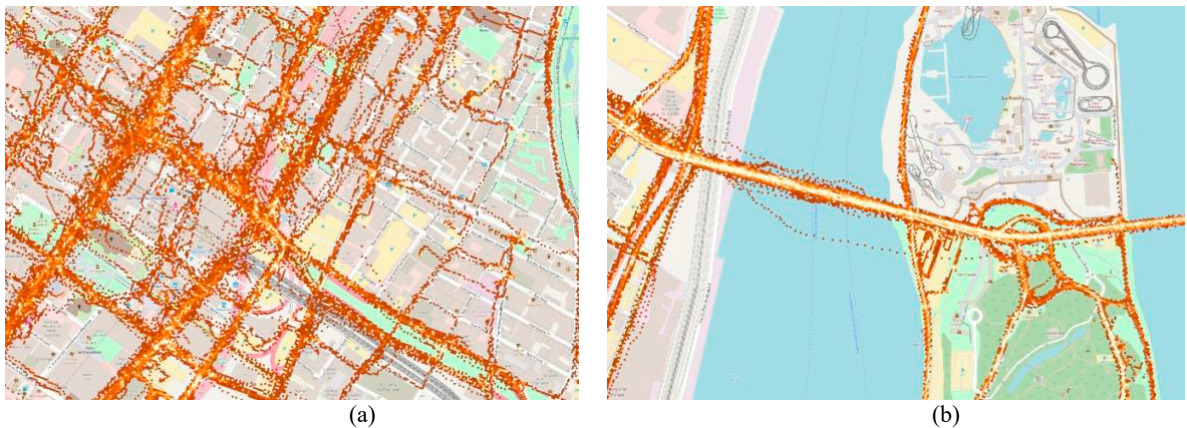
Fig. 1. Typical GNSS data quality for an urban canyon (a) and bridge (b) in Montreal, Canada
