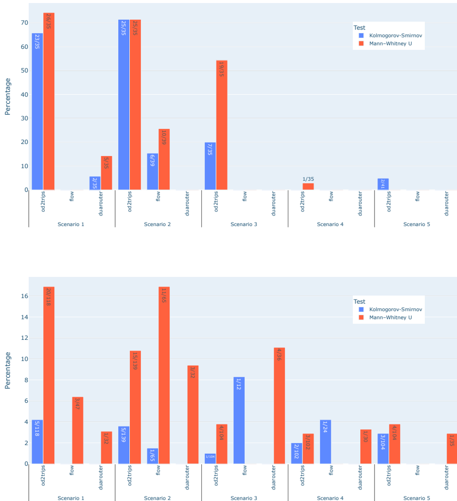
Fig. 7: Proportions of OD pairs (GNSS travel times) (top) and BT pairs (BT travel times) (bottom) for which the null hypothesis is not rejected with a 5 % type I error rate (the number of non-rejected tests over the total number of tests are shown in the bars).
