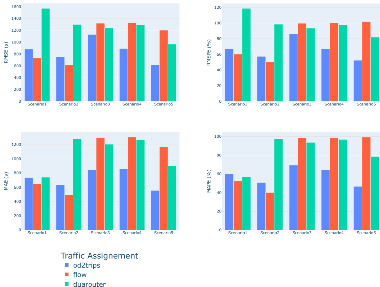
Fig. 8: RMSE, RMSPE (top), MAE and MAPE (bottom) for the OD pairs (GNSS data) per scenario and traffic assignment method.
