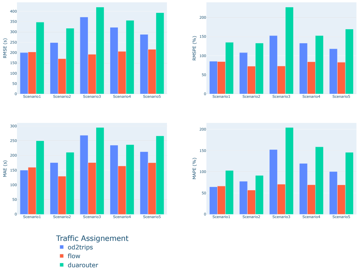
Fig. 9: RMSE, RMSPE (top), MAE and MAPE (bottom) for the BT data per scenario and traffic assignment method.
