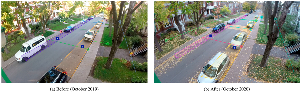
Fig. 3: The screenlines and zones before and after speed hump installation on Stuart Street
