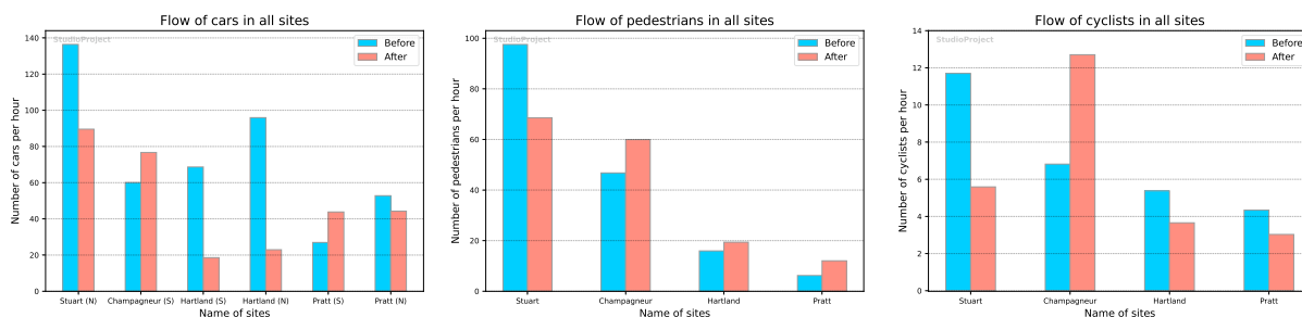
Fig. 5: Flow of street users before and after the speed humps installations
