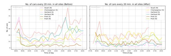
Fig. 7: Number of cars over time observed in all sites before and after the speed hump installations
