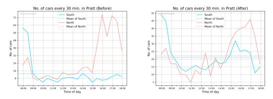
Fig. A.16: Number of vehicles in two-way streets by direction before and after speed humps installation
