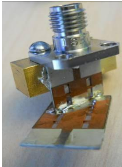
Fig. 16. Photograph of the fabricated 45 degree vertical rotated arm E-plane corner prototype.
