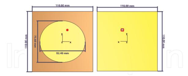
**Figure 12.**Front and back view of simulated OWPA in CST studio suite®.
