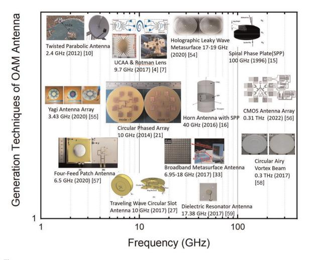
Figure 1. State-of-the-art generation techniques of OAM wave using different antenna types from GHz to THz [54-59].
