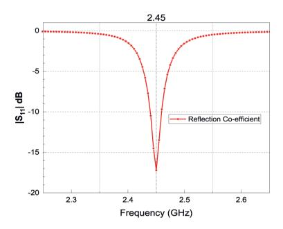
**Figure 5.**Reflection coefficient of eight-element UCAA.
