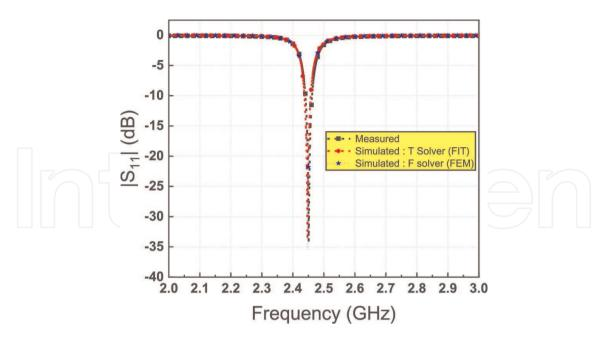
**Figure 10.**Simulated and measured reflection coefficient of PWPA.
