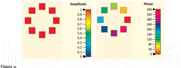
Amplitude and phase excitation pattern of an eight-element array.
