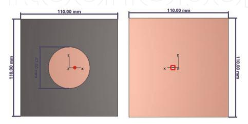
**Figure 9.** Front and back view of simulated plane wave circular patch antenna in CST studio suite®.
