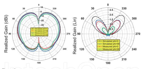
**Figure 16.**1D polar plot of simulated and measured realized gain for E-plane and H-plane: (a) realized gain in dBi and (b) realized gain in linear.
