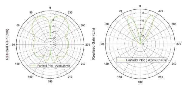
**Figure 8.**1D polar plot of gain of a UCCA antenna. (a) Realized gain (dBi) and (b) realized gain (linear).
