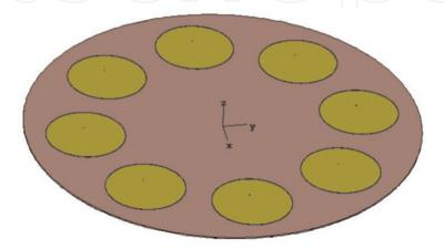
**Figure 3.** Eight-element uniform circular antenna array (UCAA) for OAM antenna design.
