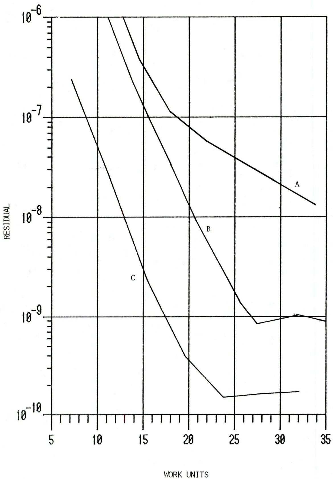
FIG. 20 EFFECT ON THE RELAXATION CONVERGENCE OF THE TOTAL NUMBER OF NODES, FOR 153(A), 561(B) AND 1105(C).
