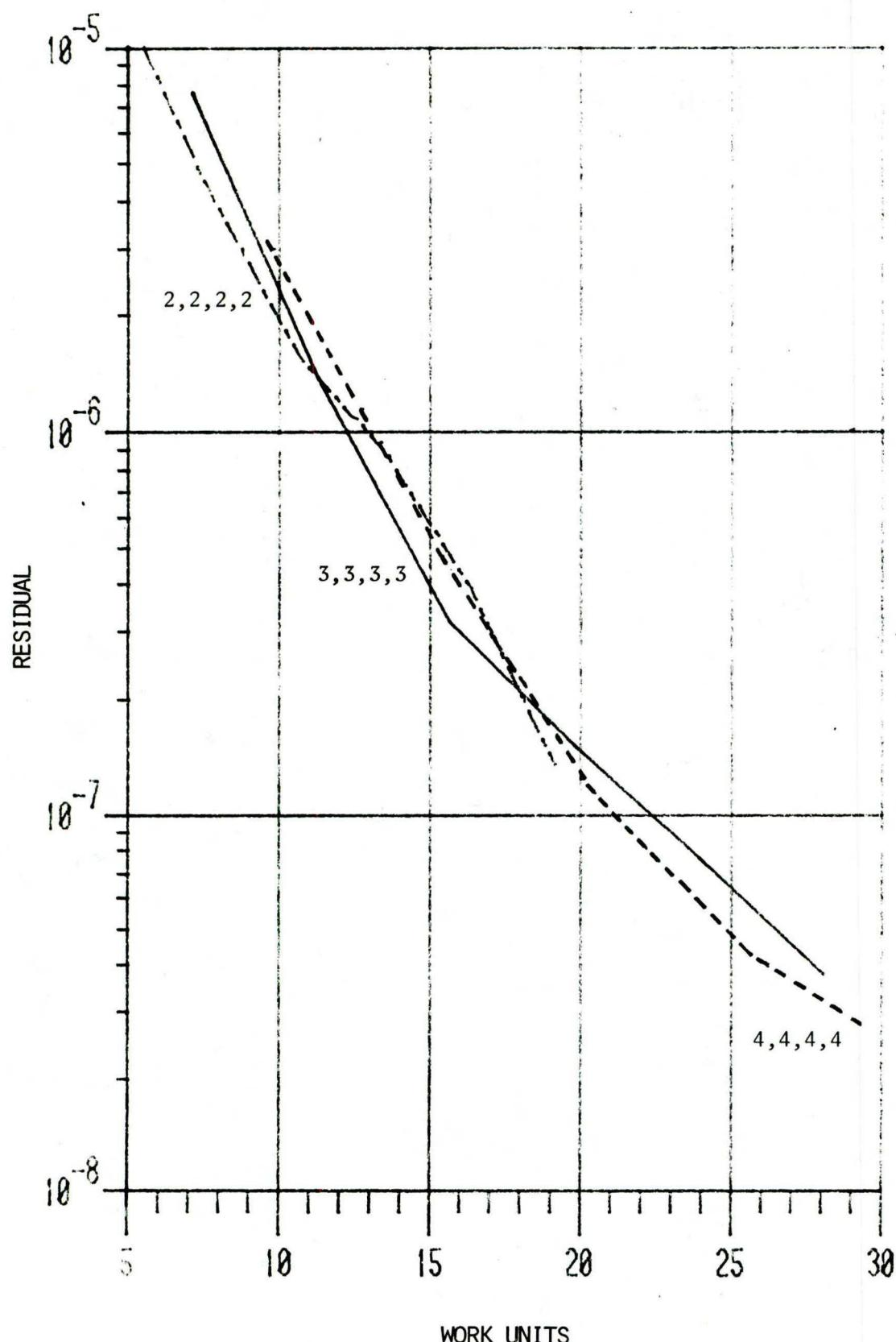
FIG. 15 OPTIMUM NUMBER OF SWEEPS PER LEVEL FOR MULTIGRID WITH LINE RELAXATION SHOWING RELAXATION HISTORIES WITH 3 AND 4 SWEEPS PER LEVEL.
