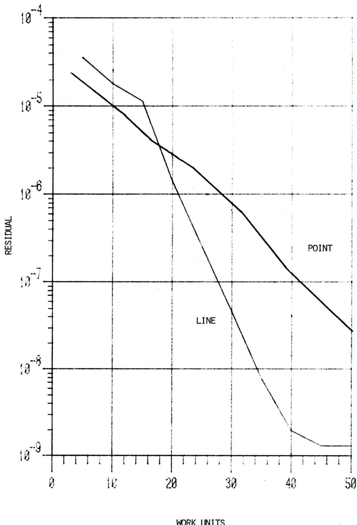
FIG. 9 COMPARISON OF OPTIMUM RELAXATIONS USING POINT AND LINE SOR FOR CASCADE B USING  $17 \times 33$ .
