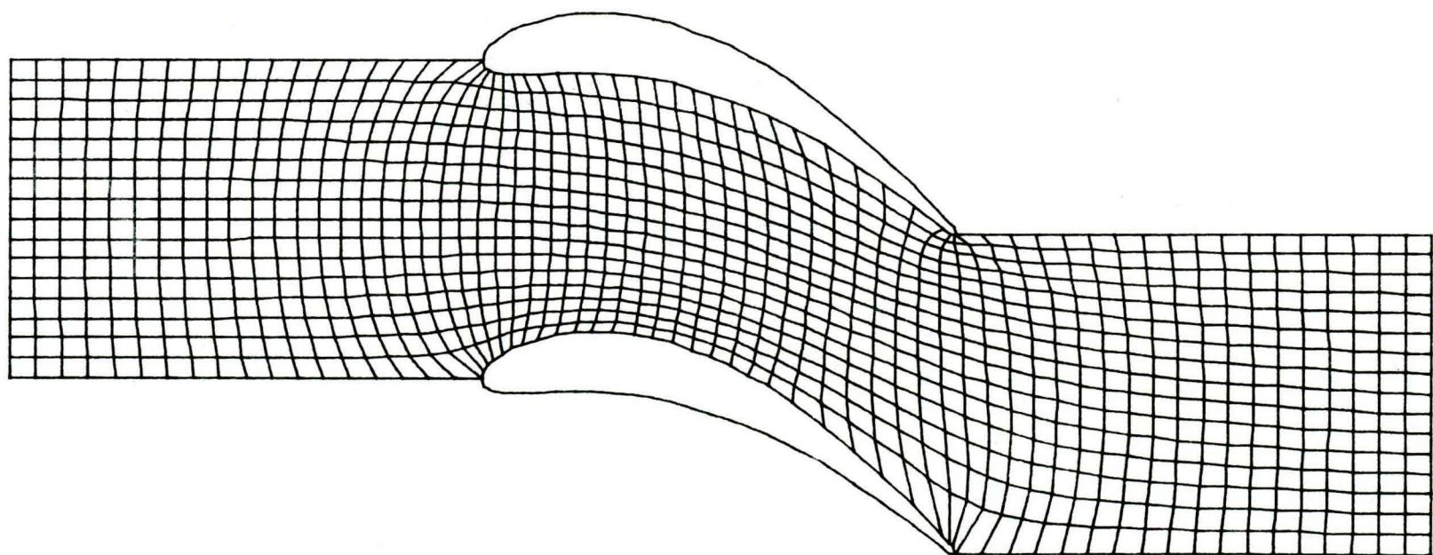
FIG. 10 BODY-FITTED COORDINATES FOR CASCADE A USING 17 x 65
