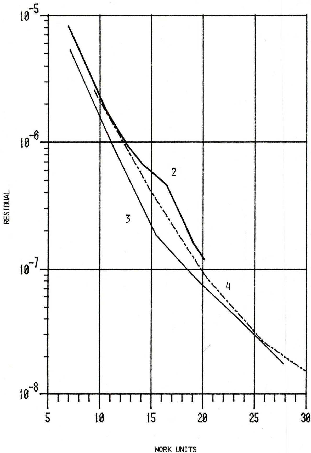
FIG. 14 OPTIMUM NUMBER OF SWEEPS PER LEVEL FOR MULTIGRID WITH POINT RELAXATION SHOWING RELAXATION HISTORIES WITH 2, 3 AND 4 SWEEPS PER LEVEL.
