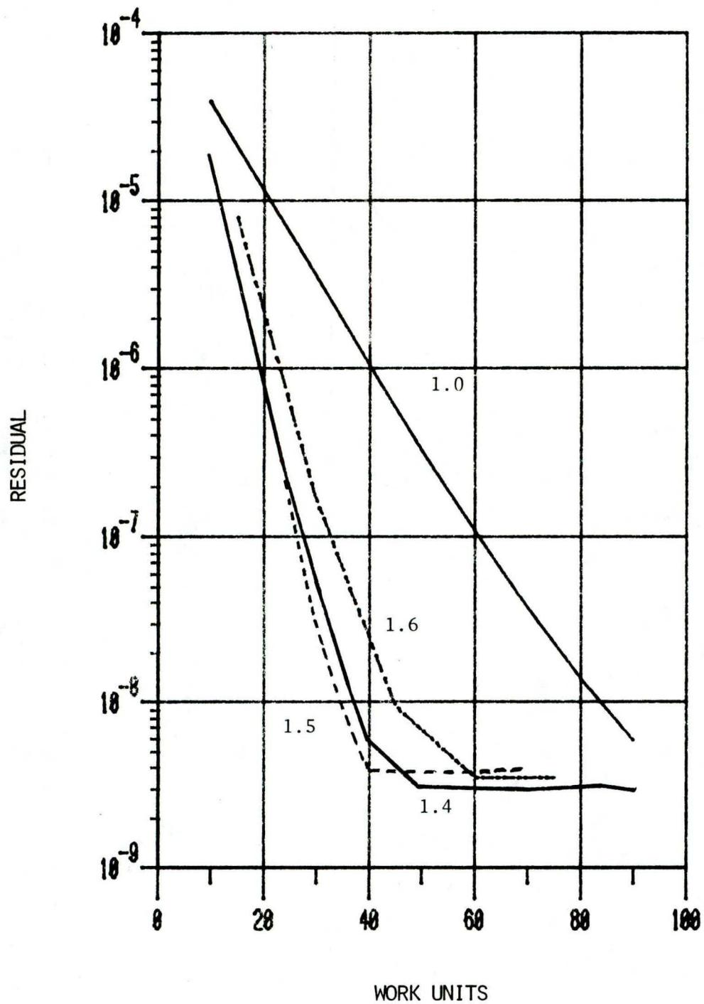
FIG. 6 OPTIMUM RELAXATION FACTOR FOR POINT SOR USING  $17 \times 33$  NODES FOR CASCADE A.
