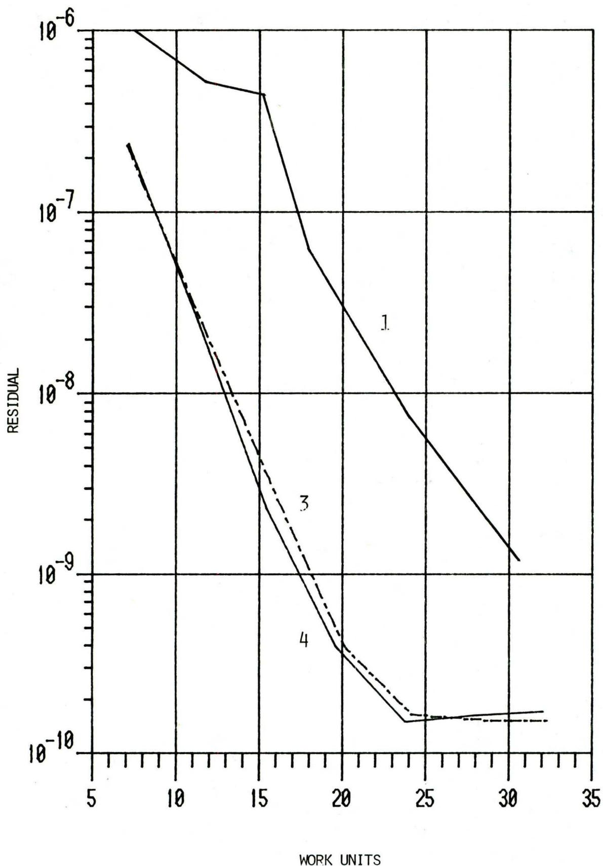
FIG. 12 COMPARISON OF RELAXATION HISTORIES USING 1, 3 AND 4. GRID LEVELS FOR LINE SOR AND MULTIGRID LINE SOR WITH THREE SWEEPS ON EACH LEVEL.
