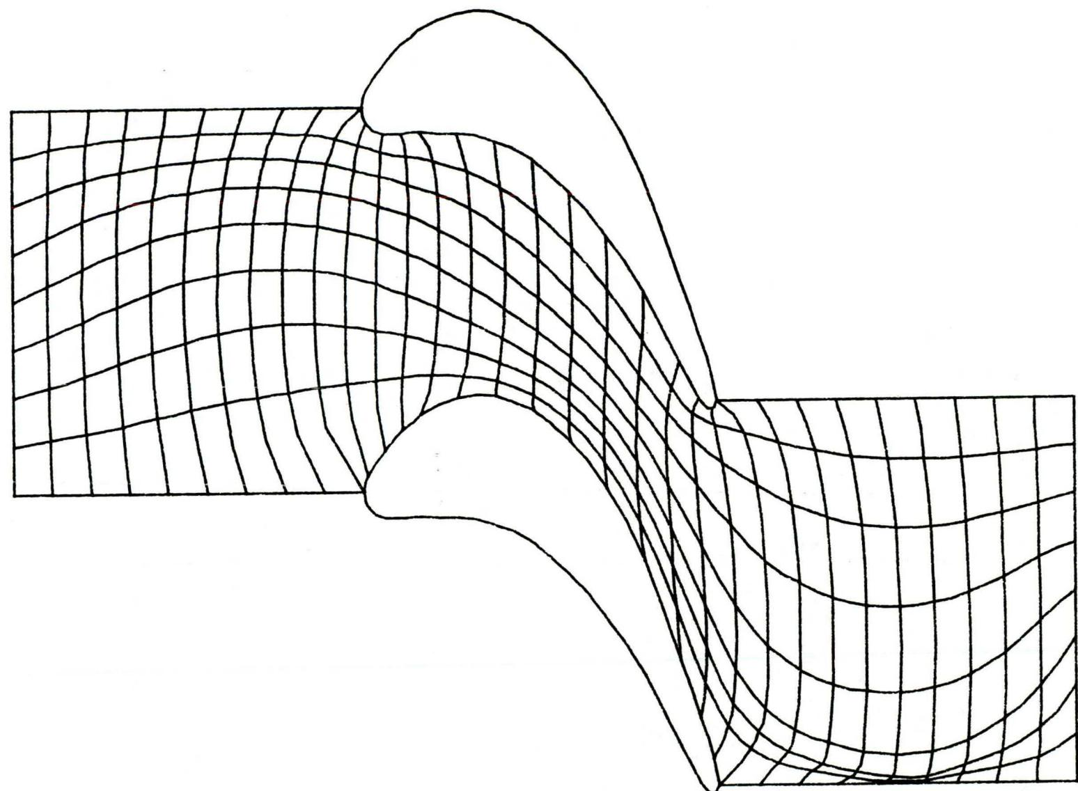
FIG. 22 ATTRACTION OF N-LINES TO TOP LEADING EDGE AND BOTTOM TRAILING EDGE, FOR CASCADE B (17 x 65).
