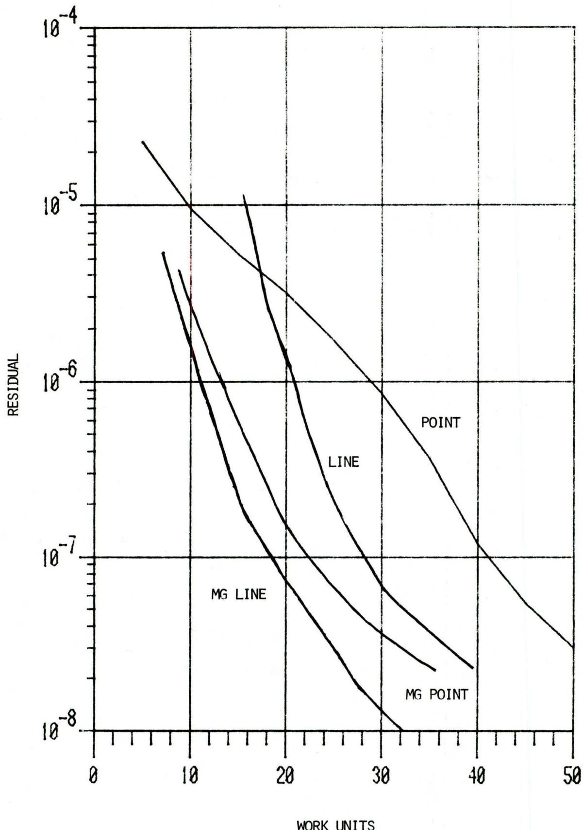
FIG. 17 COMPARISON OF RELAXATION HISTORIES FOR THE 4 METHODS FOR CASCADE A USING 9 x 17 NODES.
