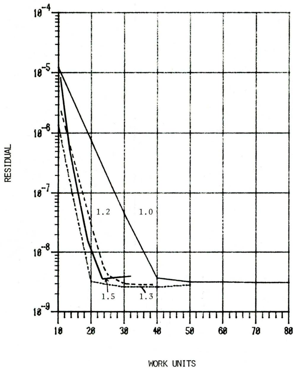
FIG. 7 OPTIMUM RELAXATION FACTOR FOR LINE SOR USING  $17 \times 33$  NODES FOR CASCADE A.
