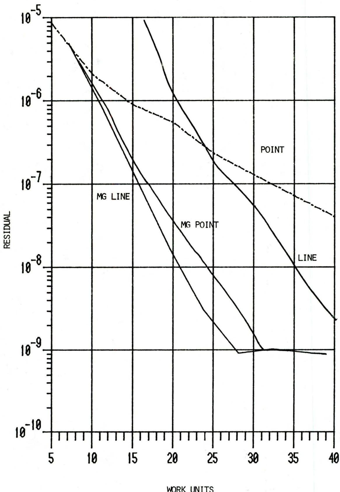
FIG. 18 COMPARISON OF RELAXATION HISTORIES FOR THE 4 METHODS FOR CASCADE A USING 17 x 33 NODES.
