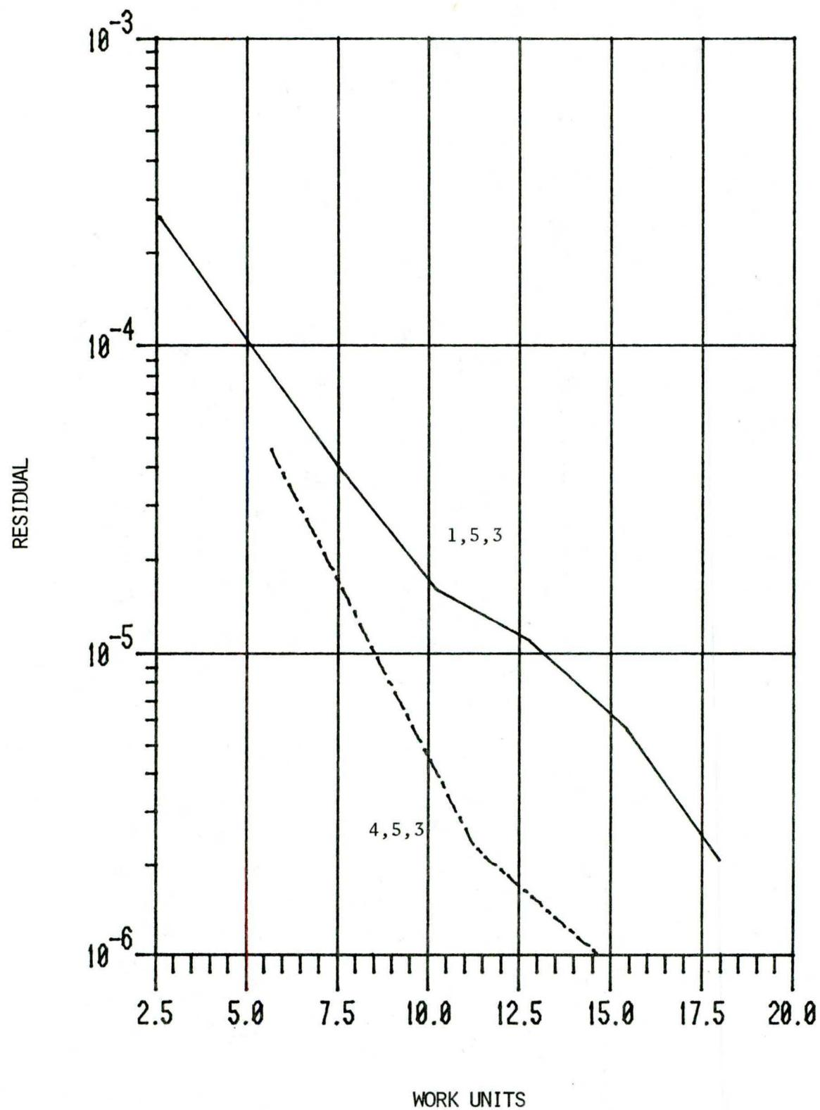
FIG. 16 EFFECT OF THE NUMBER OF SWEEPS ON THE FINE GRID ON THE CONVERGENCE RATE OF MULTIGRID WITH LINE RELAXATION.
