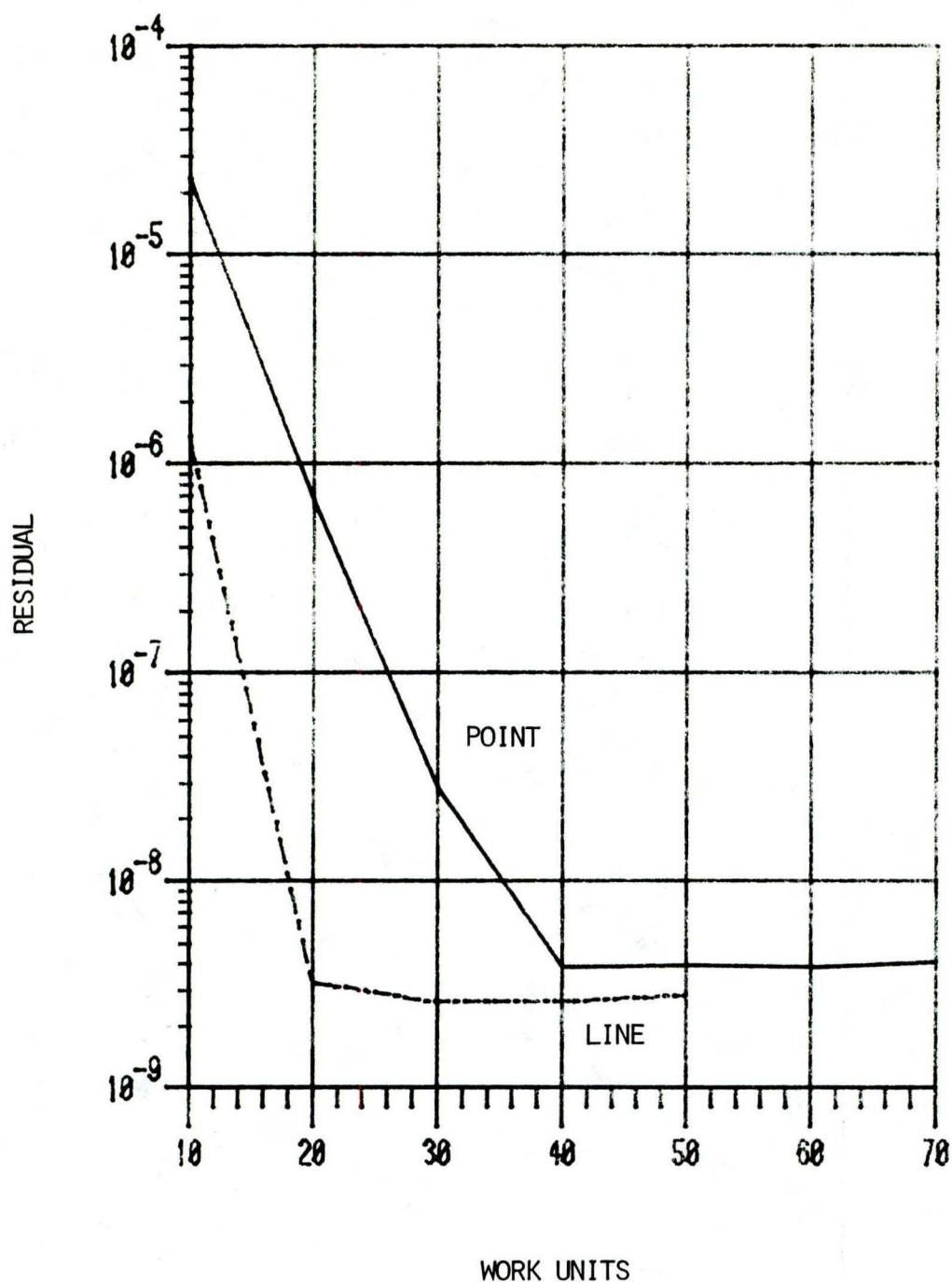
FIG. 8 COMPARISON OF OPTIMUM RELAXATIONS USING POINT AND LINE SOR FOR CASCADE A USING  $17 \times 33$ .
