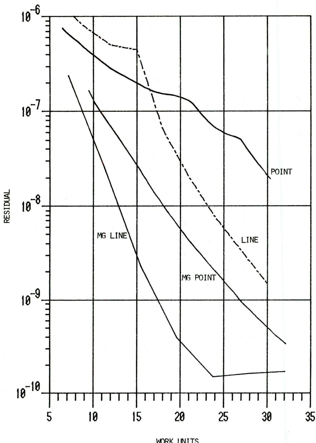
FIG. 19 COMPARISON OF RELAXATION HISTORIES FOR THE 4 METHODS FOR CASCADE A USING 17 x 65 NODES.
