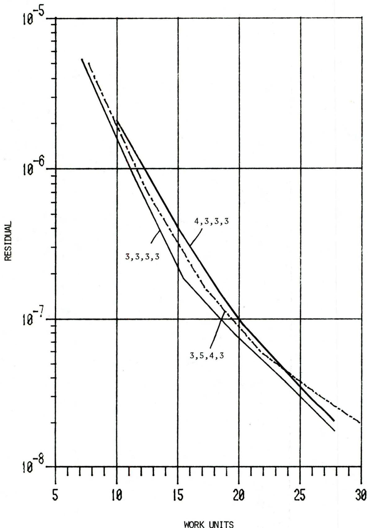
FIG. 13 COMPARISON OF RELAXATION HISTORIES OF MULTIGRID WITH POINT SOR USING 4 GRID LEVELS AND 3,3,3,3 AND 4,3,3,3 AND 3,5,4,3 SWEEPS ON THE FINE TO COARSE GRID.
