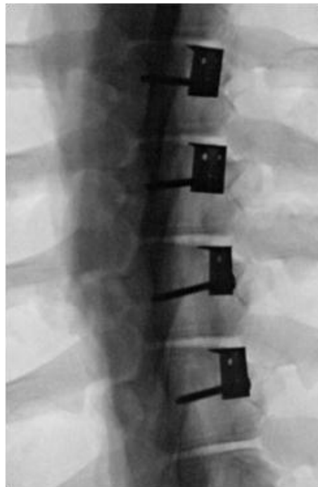
Figure 5.7: Article 4 figure 1 Fluoroscopic image of harvested instrumented porcine spine with intravertebral epiphyseal device
