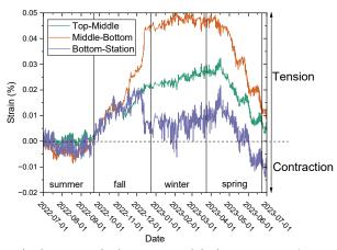
Fig. 10. Calculated strains between paired coupons, and the bottom coupon/measurement box.
