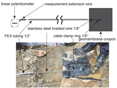
Fig. 3. Components of the geomembrane displacement measurement system.
