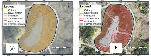
Fig. 2. Maps of the Aldermac mine waste storage area showing the comparison of the elevation contours from the as built plan (a) to the elevation contours in September 2022 (b).
