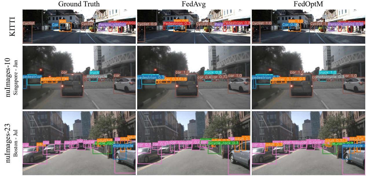
FIGURE 4.9 Qualitative results of YOLOv7 on testing data. Images are resized to the input resolution of 640px before inference, while retaining aspect ratio. The model was trained with the FedAvg baseline and the FedOptM optimized procedure on KITTI (IID) and two separate class maps of nuImages (non-IID).
