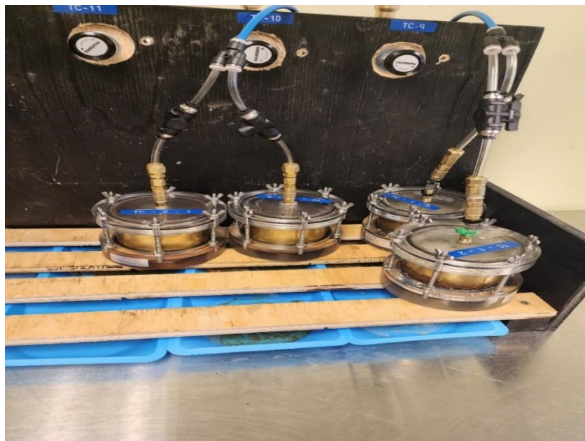
Figure 4.2 Pressure cells (Tempe cells) used to determine the WRC of tailing mixtures
