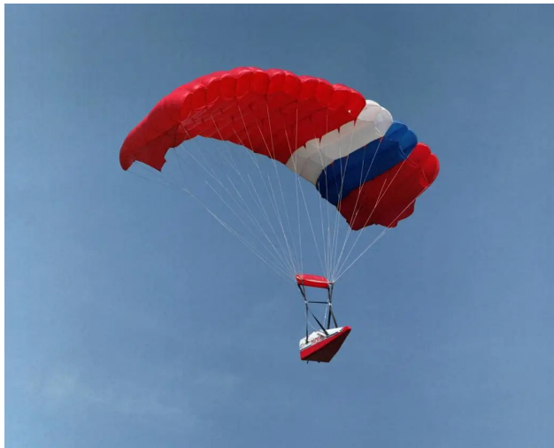
Figure 2.5 NASA's Spacewedge, an example of a parafoil-based recovery system, from [7]
