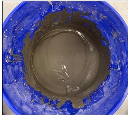
Figure 7.3: A photo of tested paste backfill at a solids content by mass of 75%
