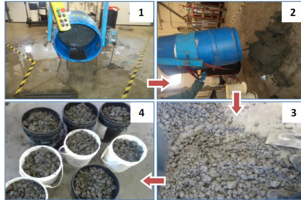
Figure 2.22: A process for preparing the paste aggregate fill (reproduced of Hane et al. 2017 with permission)
