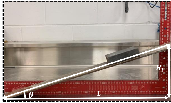
Figure 4.27: The tilt test with a steel block and a steel plate
