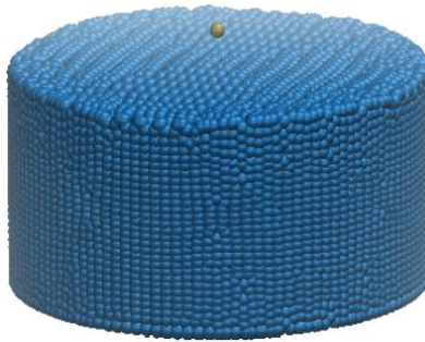
Figure 2.28: Numerical model of a single particle settling in a fluid represented by the SPH particles (reproduced of Zhu et al. 2021 with permission)
