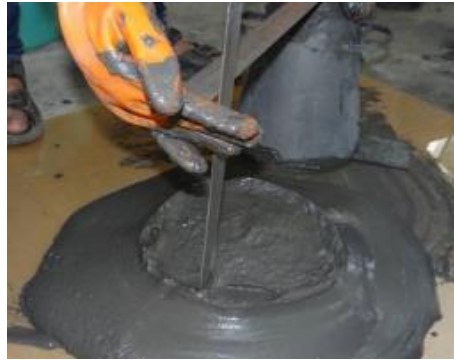
Figure 2.19: A photo of slump test to measure the yield stress of paste backfill (reproduced of Behera et al. 2020 with permission)
