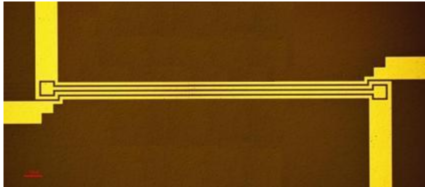
Figure 5.36 An SEM photo of the fabricated Lange coupler before bonding wires assembly.
