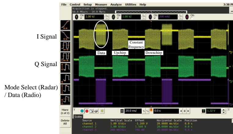
Figure 3.42 A typical waveform of the received signal for a static object.
