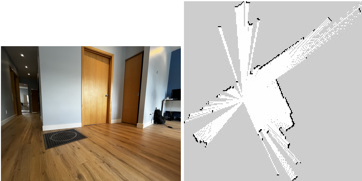
FIGURE 4.8 Example comparing the actual environment and the generated map through SLAM
