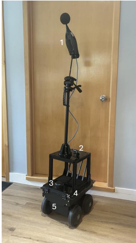
FIGURE 4.2 Proposed robotic platform. 1. Sound level meter, 2. USB camera, 3. LiDAR, 4. Rover payload with embedded NUC computer, IMU, and WiFi router, 5. Wheeled robot (Rover Robotics Mini)
