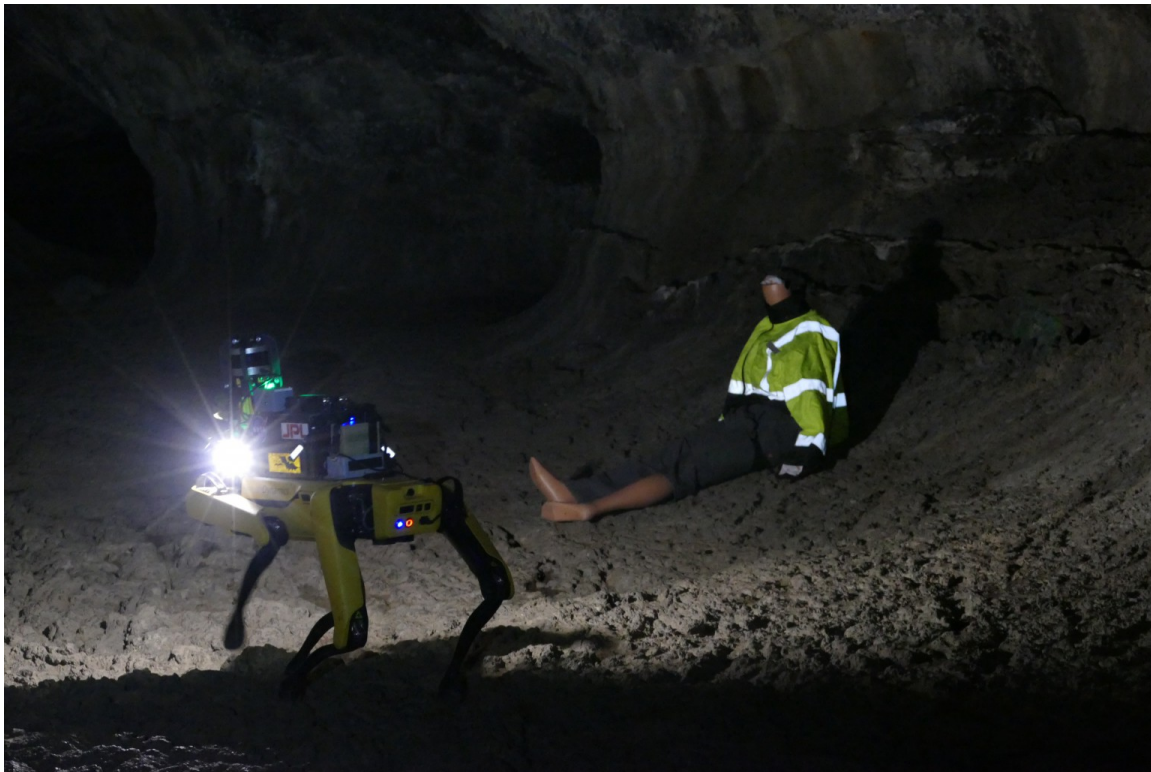
Figure 4.1 One of CoSTAR’s Spot quadruped robots deployed at Lava Beds National Monument with the NEBULA perception and computing payload on board (Credit: NASA BRAILLE)
