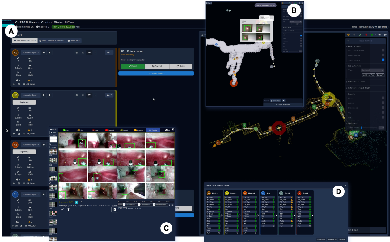
Figure 5.4 An overview of the major UI components. (A) The Robot and associated Copilot task cards. (B) The split-screen 3D visualization view with view controls, WiFi signal strength overlay, and an artifact card showing on the map. (C) The artifact drawer. (D) The robot health systems component.
