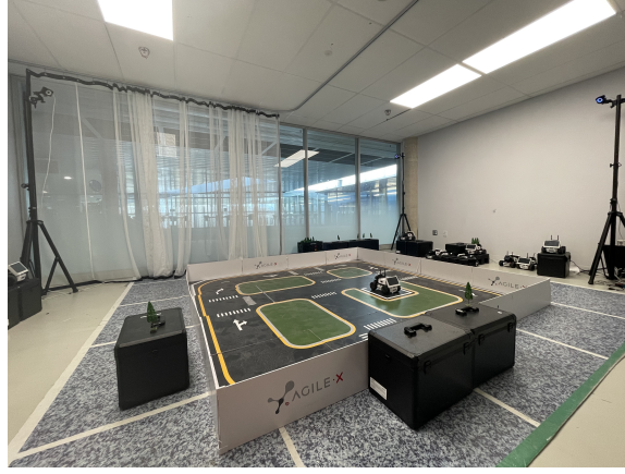
Figure 6.2 This photo depicts the real-world environment used to validate the performance of MOSEAC on the Agilex Limo. The cameras on the left, right, and middle stands are three of the four cameras comprising the OptiTrack positioning system.
