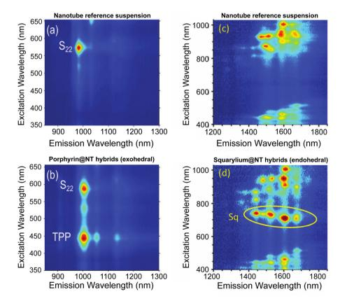
**Fig. 17** Excitation Energy transfer observed through PLE spectroscopy of functionalised SWCNTs ((b) and (d)) by comparing the PLE maps with nonfunctionalised SWCNTs ((a) and (c)). Additional bands can be clearly observed, corresponding to specific absorption of the adsorbed (b) and encapsulated (d) dye molecules and emission from the SWCNTs. Adapted with permission from ref. 212 and 209.
