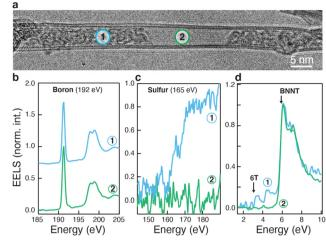
**Fig. 22** (a) HRTEM image of a partially filled 6T@BNNT suspended on a Molybdenum-SiO<sub>2</sub> TEM grid. (b) and (c) Chemical analysis of selected areas (1) and (2) in (b) using core-loss STEM-EELS at the boron K-edge (192 eV) and sulfur L2,3-edge (165 eV). (d) Measurements of the energy levels in the same two areas by STEM-EELS in the 1–10 eV energy range. Data reproduced with permission from Allard *et al., Adv. Mater.* 2020, **32**(29), 2001429, Copyright 2020 Wiley.<sup>243</sup>
