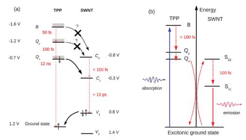
Fig. 16 Scheme use to show possible energy transfer mechanisms (a) in an electronic description through double electron transfer, (b) in an excitonic description.
