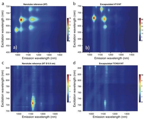
Fig. 15 PLE map: PL signal intensity *versus* emission (x-axis) and excitation (y-axis) of NT09 (a), 4T@NT09 (b) NT09 (c) and TCNQ@NT09 (d), Note that here the intensities have been normalized by adjusting the absorption intensity on the  $E_{22}$  transitions of both samples.
