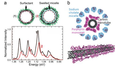
**Fig. 5** (a) Swelling of the hydrophobic core of the micelle surrounding a SWCNT (up) NIR fluorescence spectra of an sodium dodecylbenzene sulfonate (SDBS)-coated SWCNT suspension after addition of *o*-dichlorobenzene (ODCB) (bottom), adapted with permission from *J. Am. Chem. Soc.* 2008, **130**(48), 16330–16337, Copyright 2008 American Chemical Society.<sup>33</sup> (b) Schematic representation of the micelle wrapped and functionalized compounds, side and 3D views.
