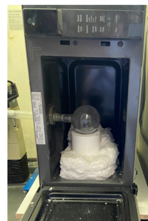
Figure 1. Experimental setup: (a) MW pyrolysis setup and (b) microwave cavity interior.
