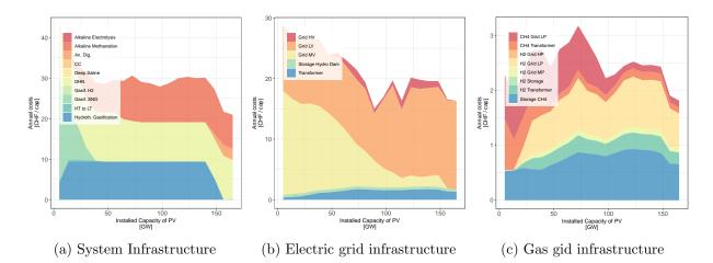
**Figure 6.** Evolution of the sectors' cost composition of the Swiss energy system according to the parametrization of PV installations.
