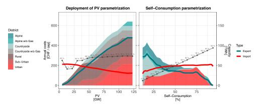
**Figure 7.** Evolution of PV LV district investments and district electricity import/export for the Swiss energy system according to PV installation and self-consumption parametrization. The points with the gray line represent the systemic decentralized PV self-consumption. The case study represents the economic optimization of a neutral (no net emission) and independent (no import) Swiss energy system in 2050 for a population of 10 Million.
