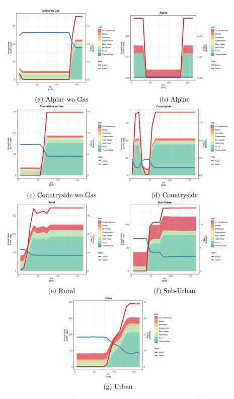
**Figure A6.** Evolution of energy system districts' cost composition of the Swiss energy system according to PV installation parametrization.
