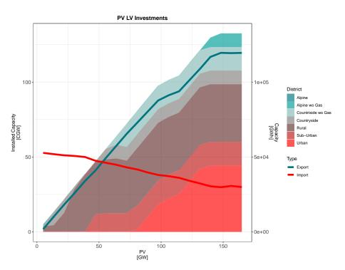
**Figure A4.** Evolution of district PV evolution of the Swiss energy system according to the PV installation parametrization. Case study of the economic optimization of a neutral (no net emissions) and independent (no imports) Swiss energy system in 2050 for a population of 10 Million people.
