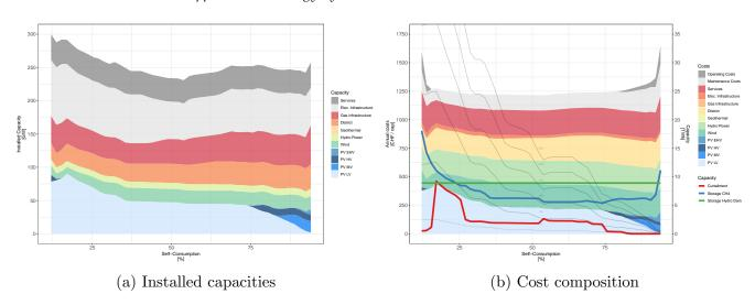
**Figure A11.** Evolution of energy system composition of the Swiss energy system according to the self-consumption parametrization. Case study of the economic optimization of a neutral (no net emissions) and independent (no imports) Swiss energy system in 2050 for a population of 10 Million people.
