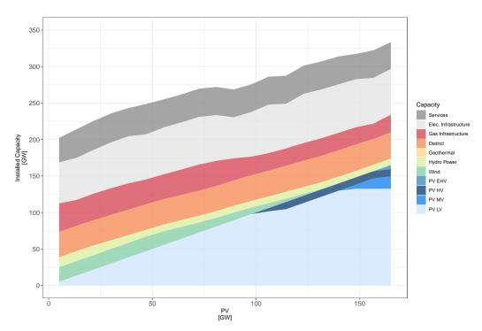
**Figure A5.** Evolution of energy system composition of the Swiss energy system according to PV installation parametrization. Case study of the economic optimization of a neutral (no net emissions) and independent (no imports) Swiss energy system in 2050 for a population of 10 Million people.
