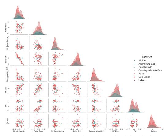
**Figure 3.** Parity plot of the investment cost of the district technologies for each identified configuration across all districts. The investment costs of each technology are normalized, assuming a Gaussian distribution for each district as the scale of the districts ranges from 1 to 244 buildings.
