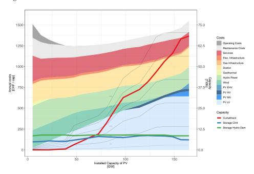
**Figure 5.** Evolution of energy system costs' composition and storage capacities of the Swiss energy system according to PV installation parametrization. The transparent lines represent the annual PV LV production fractions, allowing us to compare them with the curtailment depending on the installed PV capacity. The case study represents the economic optimization of a neutral (no net emission) and independent (no import) Swiss energy system in 2050 for a population of 10 Million.
