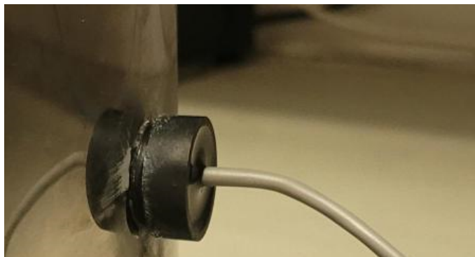
Figure 1. Photograph of H2KMPYA1000600 ultrasonic transducer attached to the stainless-steel reactor.
