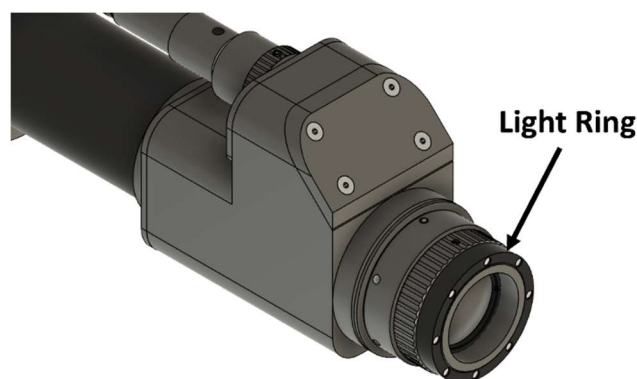
Figure 8-3 : Proposed LED ring light location at the tip of the imaging probe for near vertical bright field illumination.
