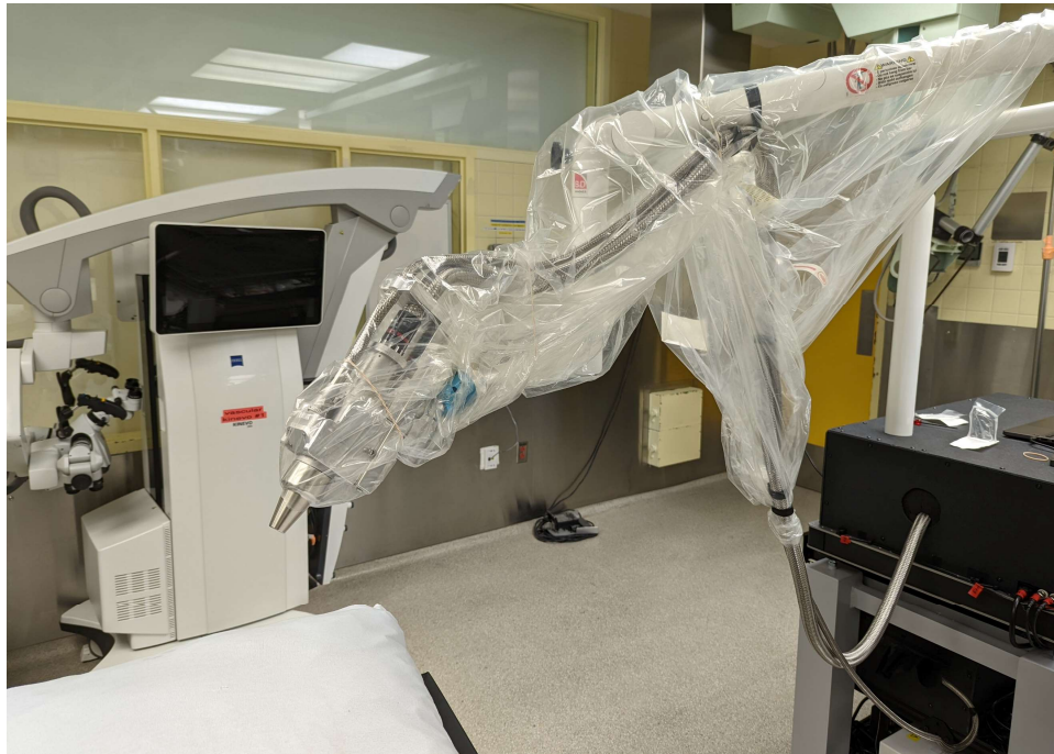
Figure 5-8 : Raman imaging probe in a clinical setting with a sterile drape covering the probe body and the articulated arm. The surgical drape is secured using sterile rubber bands and sterile tape. The probe muzzle is sterilized, ready to be inserted in a patient surgical cavity and it presents a minimal infection risk to the patient.
