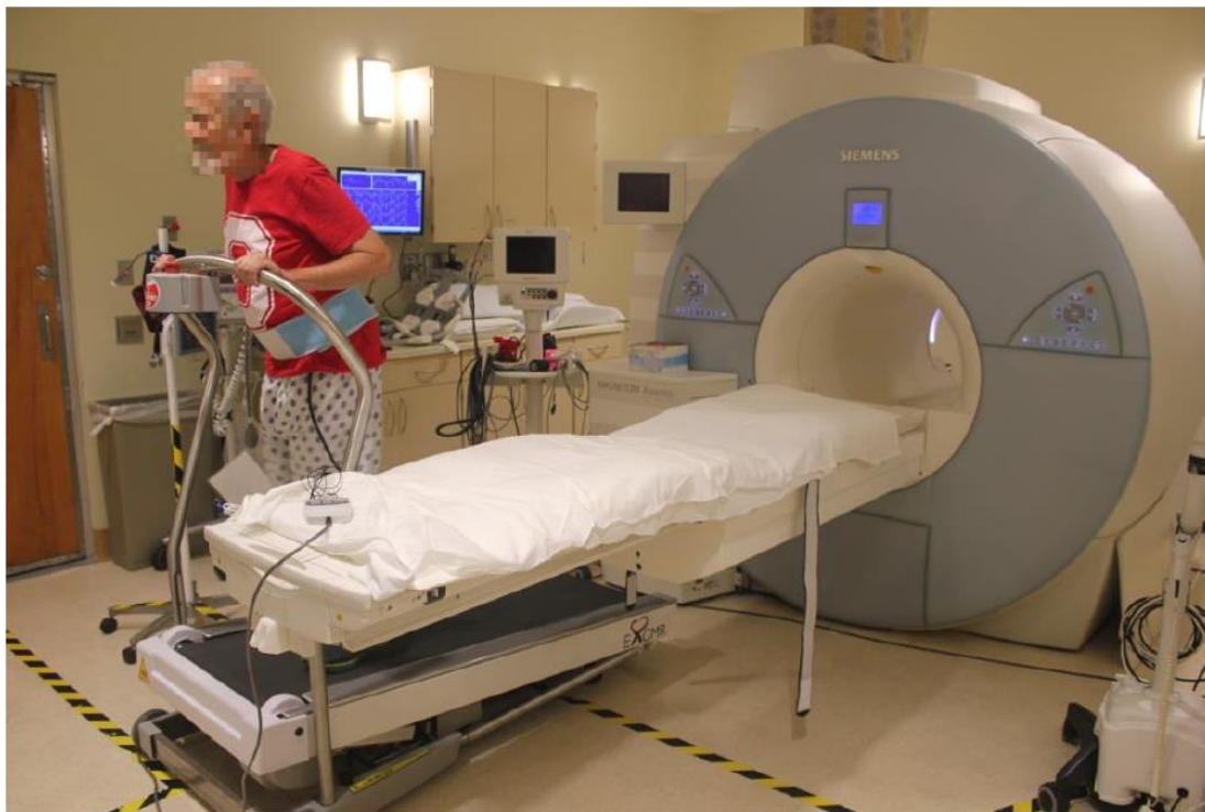
Figure 2.4 MRI-compatible scanner adjacent to a treadmill [14].
