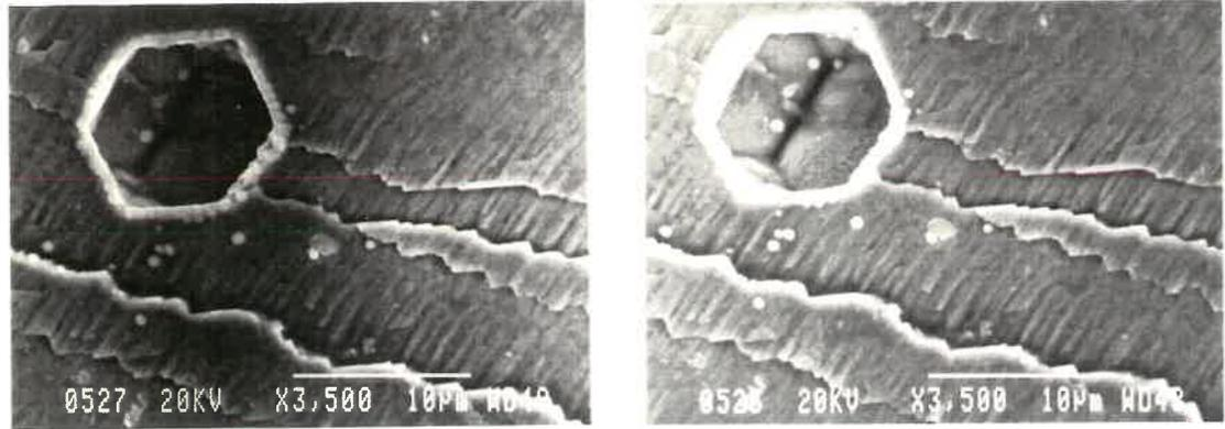
**Fig. 5.12:** Stereo pairs shows  $\{110\} \langle 100 \rangle$  cracking crystallography identified on TSCC facets produced in the region corresponding  $K \approx 15 \text{ MPa m}^{1/2}$ .
