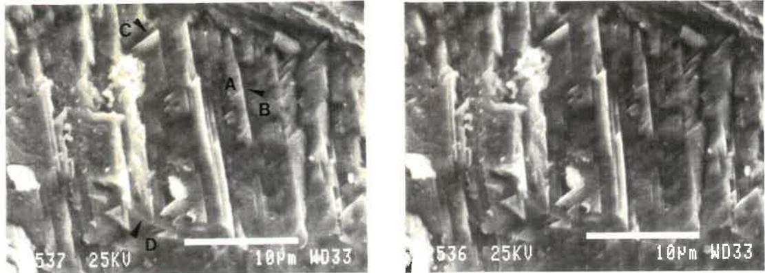
**Fig. 5.9:** Stereo pairs shows complex aspect with presence of four sets of  $\{111\}$  microfacets observed on TSCC of  $\alpha$ -brass ( $K \approx 20 \text{ MPa m}^{1/2}$ ).
