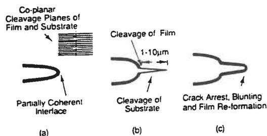
**Fig. 1.14:** Schematic diagram illustrating a film-induced cleavage model proposed for TSCC in copper and  $\alpha$ -brass by Newman et al. (202).
