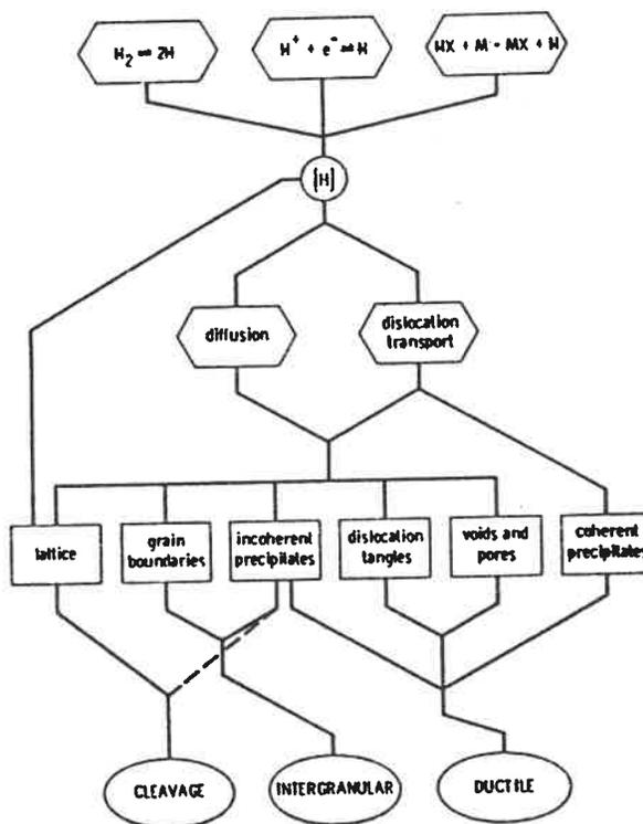
**Fig. 1.23:** Summary of hydrogen processes: sources leading to hydrogen in solution, transport leading to accumulation at microstructural locations, and finally fracture. Dashed line refers to cleavage of hydrides. From Thompson and Bernstein (264).
