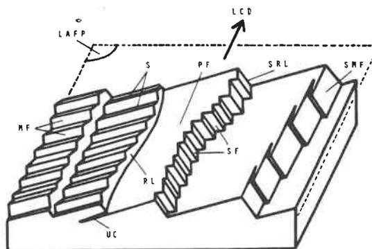
**Fig. 4.3:** Schematic diagram defining the fractographic features associated with TSCC: LAFP, local average fracture plane; LCD, local crack propagation; MF, microfacet; PF, primary facet; RL, river line; S, striations; SF, serration facets; SMF, sheet-like microfacets; SRL, serrated river line, UC, undercutting (415).
