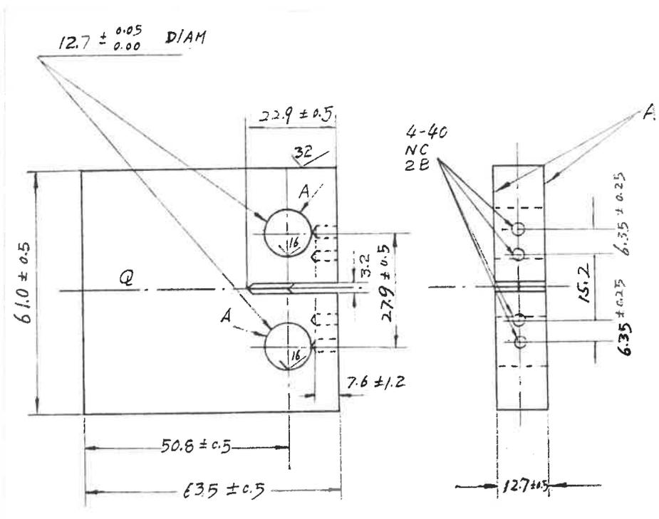
**Fig. 3.3:** Geometry of CT specimen
