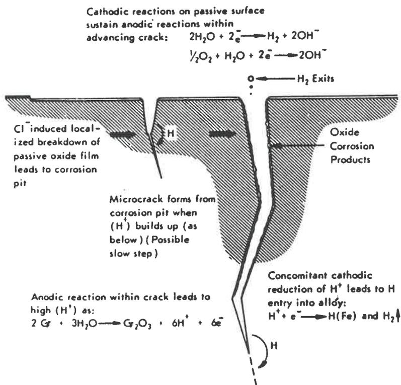
**Fig. 1.19:** Generalized model for crack initiation and propagation in SCC (the details here are for austenitic stainless steel in a chloride environment) (264).
