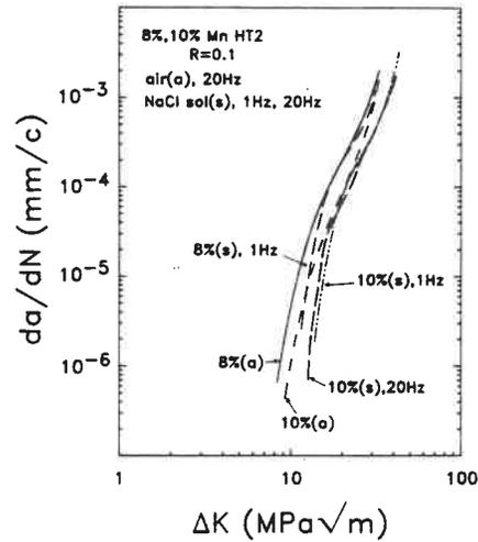
**Fig. 6.5:** Comparison of different crack propagation curves for the 8 and 10% Mn HT2 alloys.
