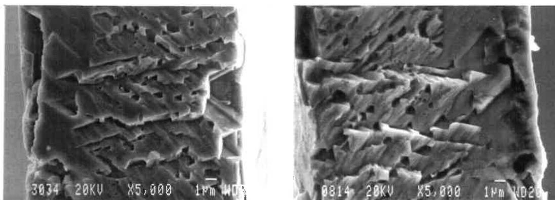
**Fig. 5.26:** Matching fracture surfaces for crystallographic cracking observed after fracture of a ribbon specimen, rinsed and dried after immersion and then fractured. Initiation occurred along a dissolution slot; cracking then followed large  $\{111\}$  facets and then two alternating sets of  $\{111\}$  microfacets.
