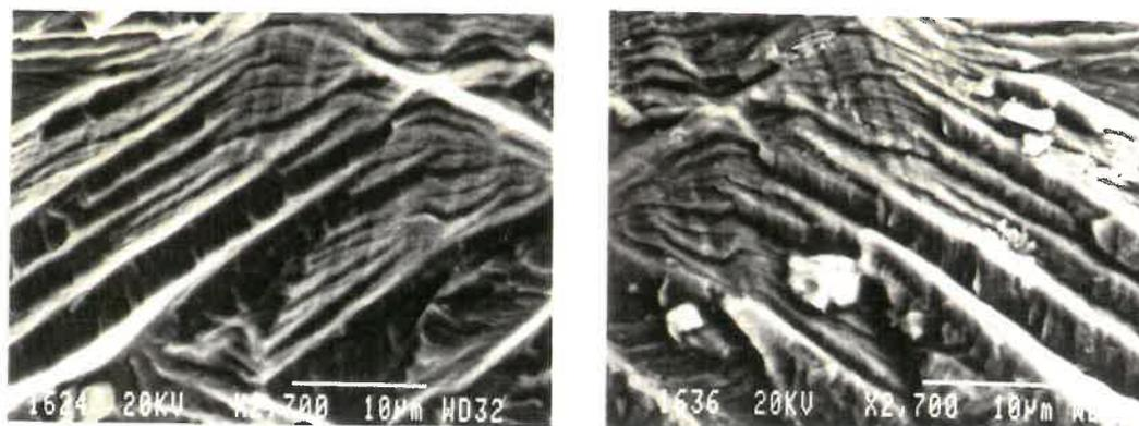
**Fig. 4.20:** The same site of the fracture surface observed on opposite fracture. The microfractographic features match in an interlocking manner.
