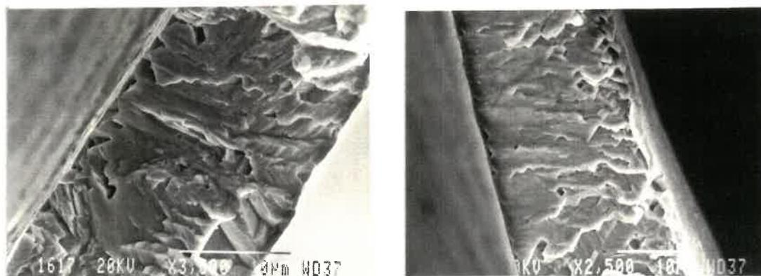
**Fig. 5.27:** Crystallographic cracking initiated at lines of the etch pits and propagated on two or more sets of  $\{111\}$  facets decohesion observed on the specimens rinsed after 100 minutes of immersion and then fractured in air.
