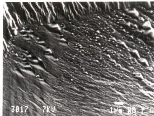
**Fig. 3.47:** Tetrahedra-like small facets present on the intergranular facets for 316 stainless steel tested in air at low  $da/dN$  values ( $\sim 10^{-6}$  mm/cycle). Very fine river lines can also be clearly seen on the intergranular facets.
