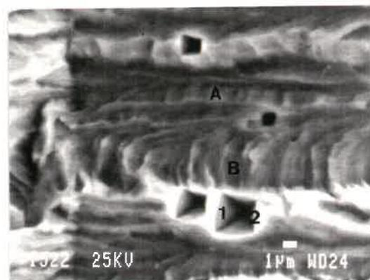
**Fig. 4.9:** Stereographic pair of micrographs from the region below the annealing twin in Fig. 4.8, allowing one to observe the microfractographic aspects at higher magnification. The presence of different sets of  $\{111\}$  microfacets can be identified. Fig. 4.9 is rotated almost  $90^\circ$  with respect to Fig. 4.8.
