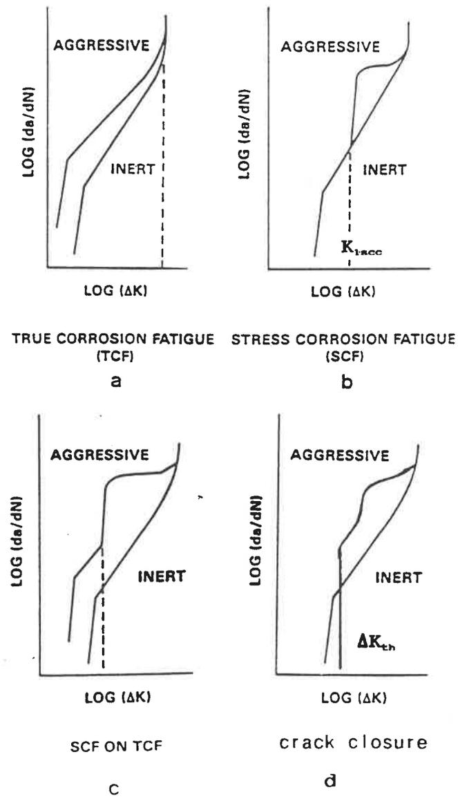
**Fig. 1.27:** Illustration of the four types of corrosion fatigue crack propagation curves (152).
