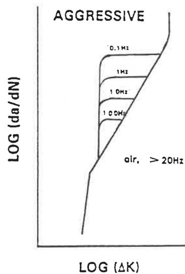
**Fig. 1.28:** Illustration of typical effect of testing frequency on corrosion-fatigue crack propagation (152).
