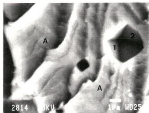
**Fig. 4.5:** Stereographic pair of micrographs showing fine striations which, in region "A" can be seen to result from the presence of sets of {111} microfacets parallel to sides 1 and 2 of the etch pits.
