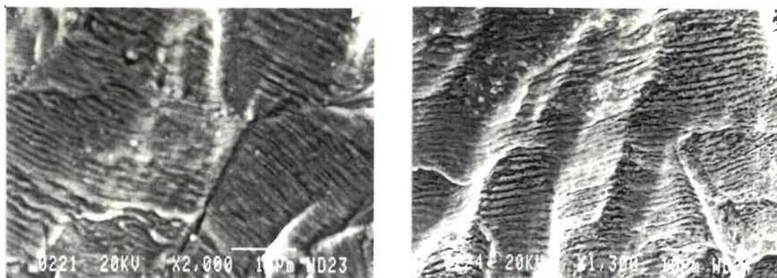
**Fig. 6.15:** Striations which cross boundaries between  $\alpha$  grains with no apparent difficulty, 8% Mn AC alloy tested at 1 Hz in the NaCl solution,  $da/dN \approx 10^{-3}$  mm/cycle.
