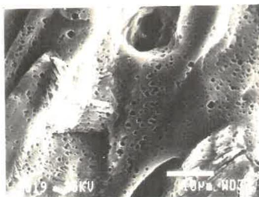
**Fig. 3.34:**  $\{111\}$  facets seen in region A of this micrograph of a near-threshold fracture surface of 2024-T351 Al alloy tested in air.
