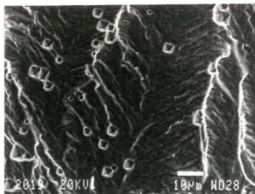
**Fig. 4.15:** Herring-bone patterns of river lines observed at quite low K. The  $\{100\}$  primary facet presents two sets of  $\{100\}$  river lines and a  $\langle 110 \rangle$  central spine.
