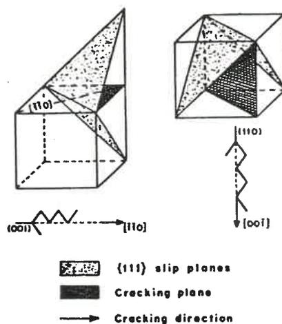
**Fig. 3.42:** Model for cracking along  $\{100\}$  or  $\{110\}$  by decohesion along two alternating  $\{111\}$  slip planes.
