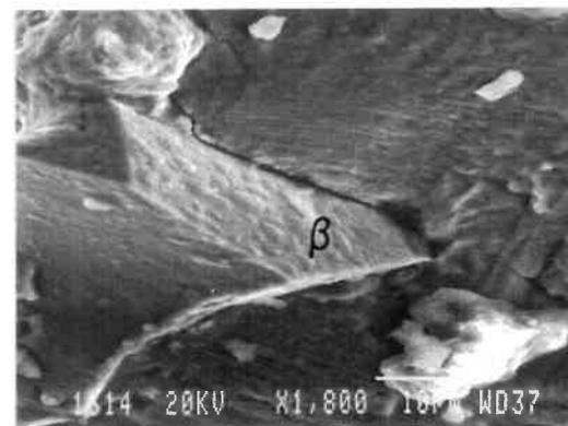
**Fig. 6.32:** (Left) Dimples in the  $\beta$  phase of the 10 % Mn HT2 alloy tested in air,  $da/dN \approx 10^{-5}$  mm/cycle. (observed after etch-pitting).
