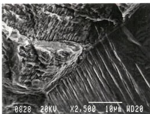
**Fig. 3.45:** Features resembling intrusions and extrusions observed on the intergranular facets for copper tested in air ( $da/dN \approx 10^{-6}$  mm/cycle).
