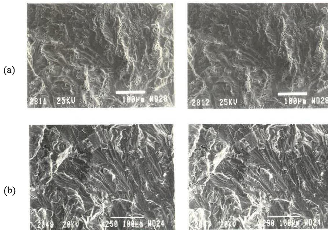
**Fig. 4.21:** Stereofractographic pairs of a relatively low magnification (a) at low and intermediate K values region, (b) at high K values region.
