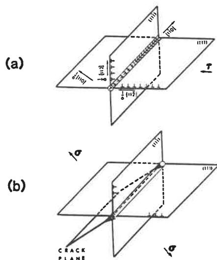
**Fig. 1.18:** Crystal geometry of the slip planes, the Cottrell-Lomer dislocation barrier and their relation to the cracking plane (163).
