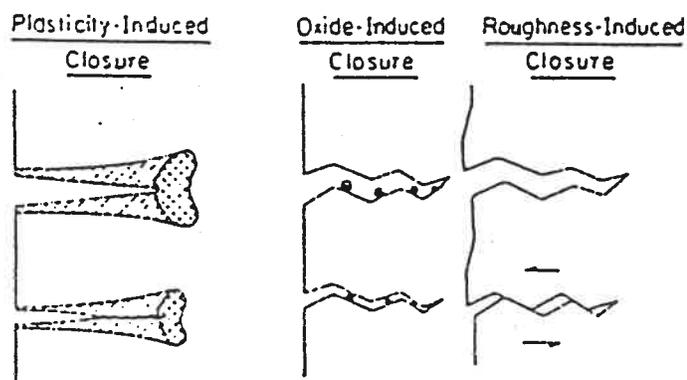
Fig. 1.4: Schematic illustration of mechanisms of fatigue crack closure (40).
