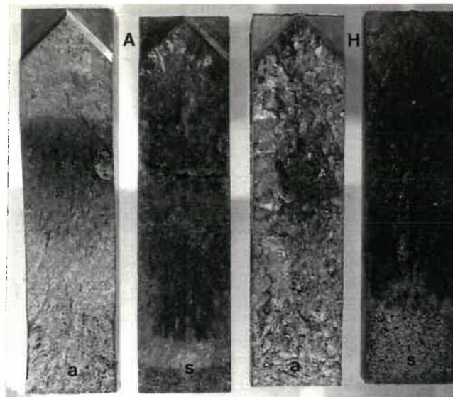
**Fig. 6.8:** Macroscopic aspect of fracture surfaces of the as-received (A) and HT2 (H) propeller specimens tested in air (a) and in NaCl solution (s).
