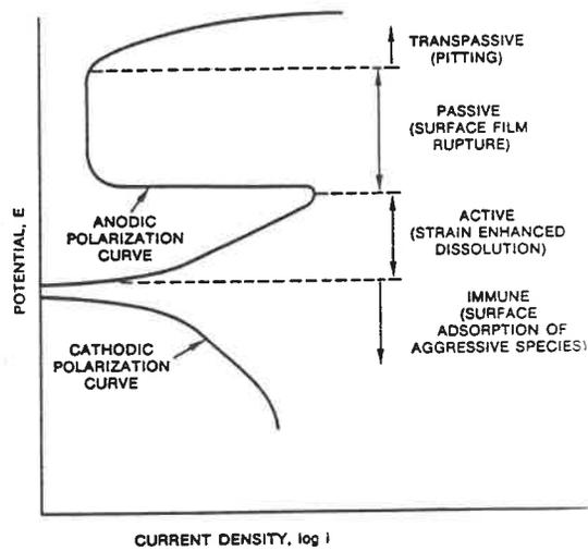
**Fig. 1.26:** Schematic of correspondence between regions of a polarization curve and corrosion fatigue mechanisms.
