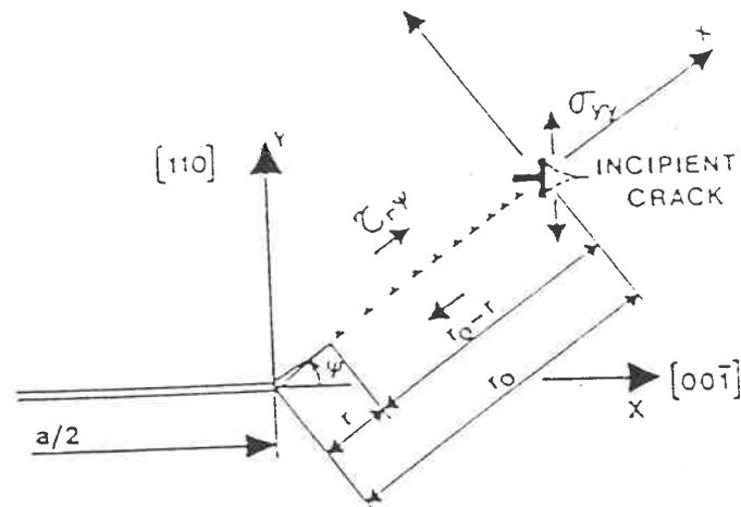
**Fig. 1.15:** Schematic drawing of a dog-leg crack, formed by corrosion along a slip plane, approaching a Lomer-Cottrell lock (model of Lichter et al. (175)).
