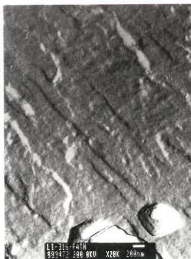
**Fig. 3.15:** Fractographic details on the near-threshold {100} average facets observed on TEM replicas.
