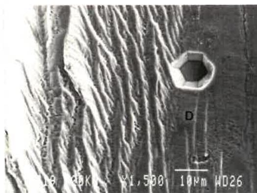
**Fig. 3.53:** Two different sets of  $\{110\}$  primary facets with  $\langle 111 \rangle$  or  $\langle 113 \rangle$  striations observed in Fe-3%Si for  $da/dN \approx 10^{-7}$  mm/cycle.
