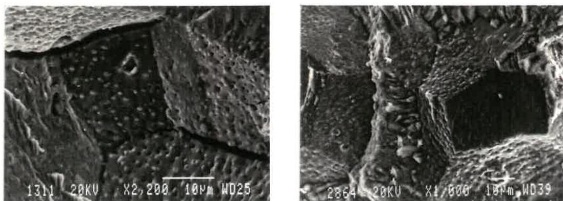
**Fig. 6.9:** Small precipitates and dimples on the intergranular-like facets produced in air for 8% Mn AC bronze at  $da/dN \approx 10^{-6}$  mm/cycle.
