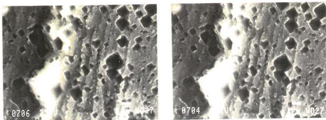
**Fig. 3.33:** Primary  $\{100\}$  near-threshold facets, with secondary  $\{111\}$  facets corresponding to serrated river lines in 2024-T351 Al alloy tested in air.
