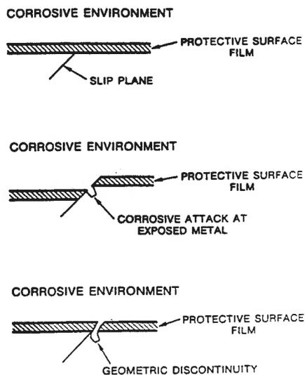
**Fig. 1.25:** Mechanism of surface film rupture for environmentally enhanced crack initiation.
