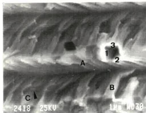
**Fig. 4.12:** The presence of an etchpit on this stereographic pair of micrographs permits one to identify the  $\{111\}$  orientations of the sheet-like microfacets. For example, the microfacets indicated A, B and C can be seen to be parallel to faces 1, 2 and 3 respectively of the etchpit.
