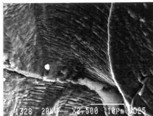
**Fig. 6.14:** Curved aspects of striations for the 8% Mn AC alloy tested in air, indicating that the cracks encounter some difficulty to cross boundaries between  $\alpha$  grains,  $da/dN \approx 10^{-3}$  mm/cycle.
