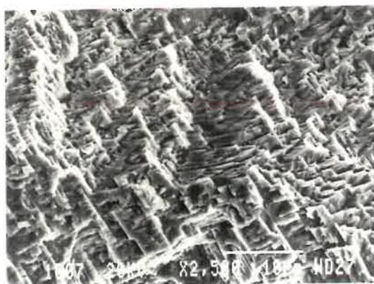
**Fig. 5.8:** Complicated fractographic aspect observed in higher K region (~ 20 MPa m<sup>1/2</sup>)
