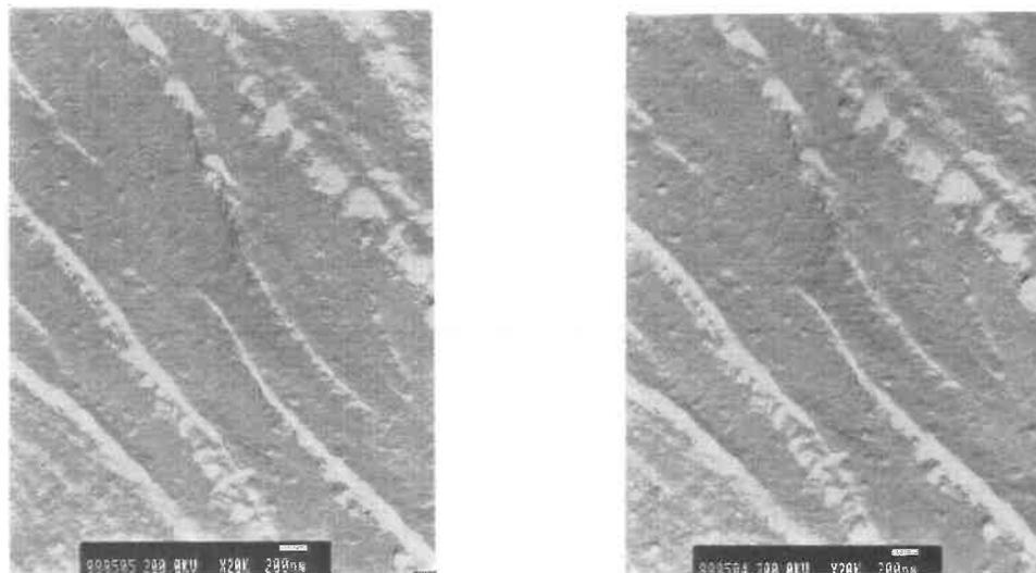
**Fig. 4.22:** Stereographic pair of TEM fractographs observed for a flat facet produced at low  $K$ .
