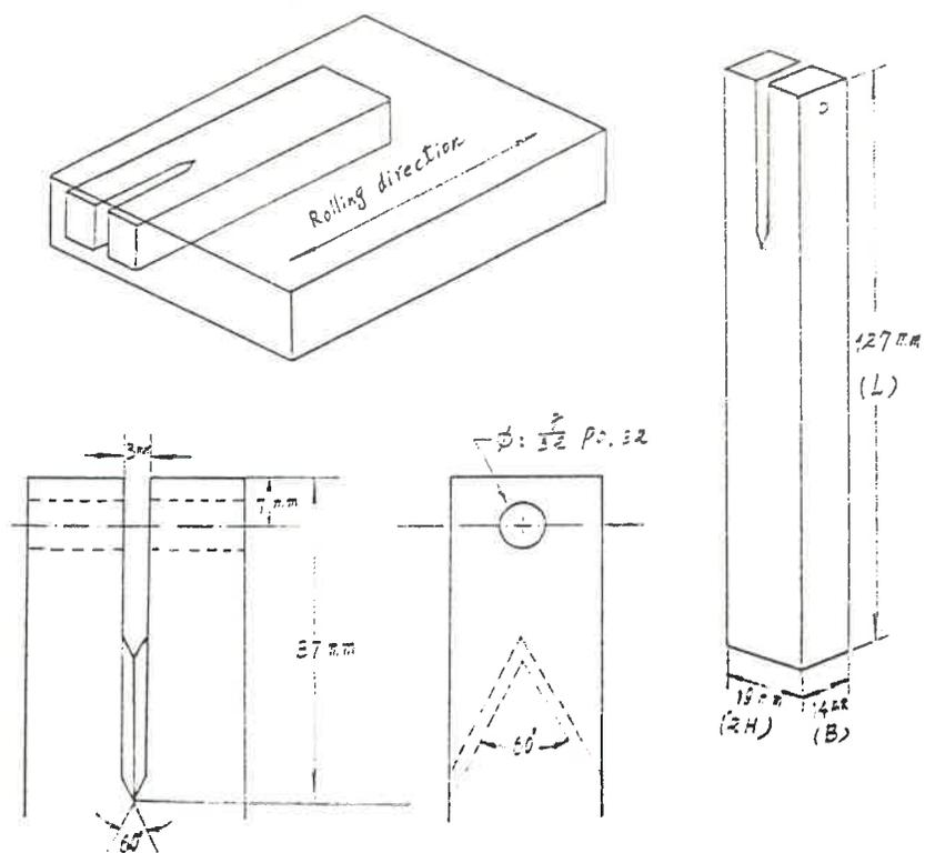
**Fig. 5.2:** Dimensions and geometry of DCB specimen.
