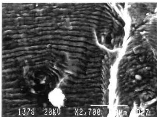
**Fig. 6.33:** Interaction of medium-size  $\kappa$  precipitates with fatigue striations in the  $\alpha$  phase, 8% Mn AC bronze tested in air,  $da/dN \approx 10^{-3}$  mm/cycle.
