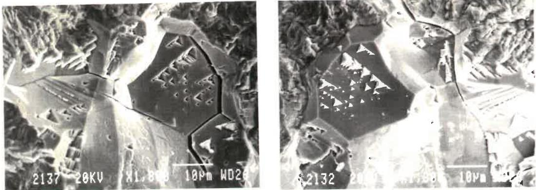
**Fig. 3.46:** Matching triangular pits and protrusions on opposite fracture surfaces of unetched intergranular facets for  $\alpha$ -brass tested in air ( $da/dN \approx 10^{-6}$  mm/cycle).
