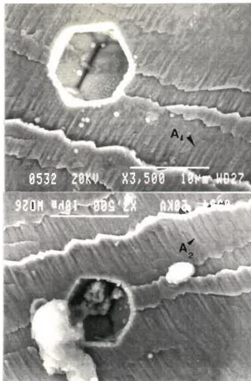
**Fig. 5.15:** The  $\{111\}$  microfacets can be seen to match in an interlocking manner. For example the facet indicated  $A_1$  matches to that indicated  $A_2$  on the mating fracture surfaces.
