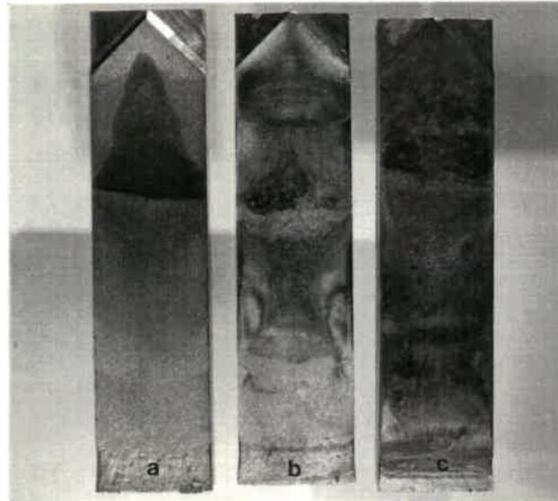
**Fig. 6.7:** Macroscopic aspect of fracture surfaces of the 8% Mn AC specimens tested in air at 20 Hz (a) and in 3.5% NaCl solution at 1 (b) and 20 (c) Hz.
