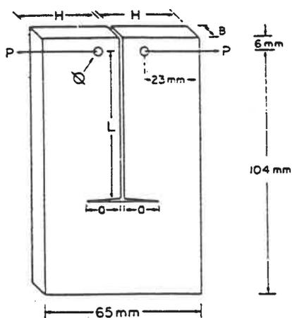
$\varnothing = 4 \text{ mm}$ ,  $P = \text{Load}$ ,  $a = \text{Crack}$
