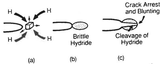
**Fig. 1.20:** Schematic illustrating a hydride-induced cleavage fracture processes.
