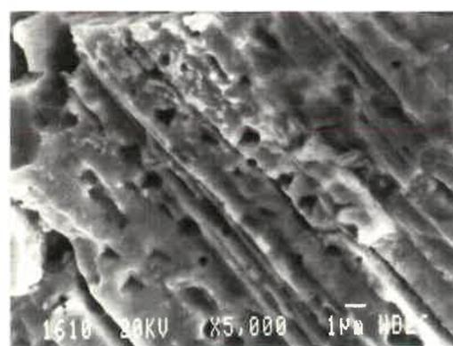
**Fig. 3.22:** Stair-like facets observed for ultra-low crack growth rates ( $da/dN \approx 10^{-8}$  mm/cycle) in 8% Mn-8% Al-2% Ni bronze tested in air (HT<sub>1</sub> condition).
