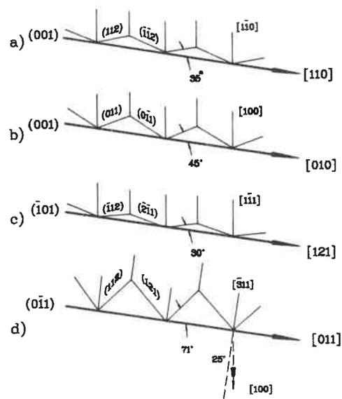
**Fig. 3.50:** Different alternate slip cracking combinations which are consistent with the experimental observations obtained on the b.c.c. metals studied.
