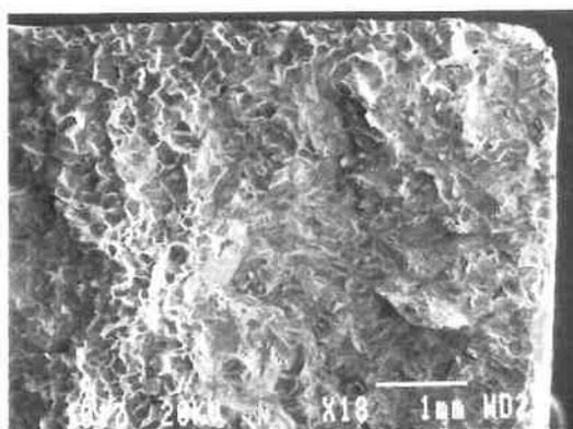
**Fig. 5.5:** Aspect of SCC of  $\alpha$ -brass viewed at low magnification
