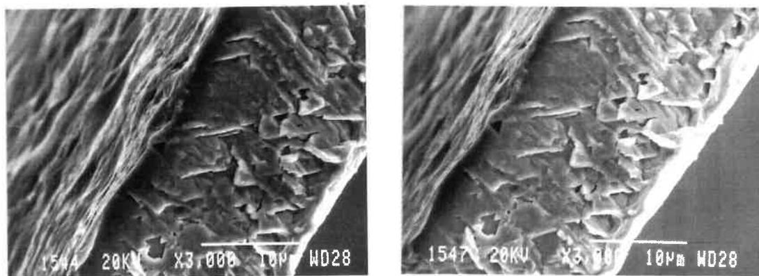
**Fig. 5.25:** Stereomicrofractographs show that crystallographic cracking initiated following the relatively large flat  $\{111\}$  facets which are almost perpendicular to the tensile axis (fractured in air after 100 minutes of immersion).
