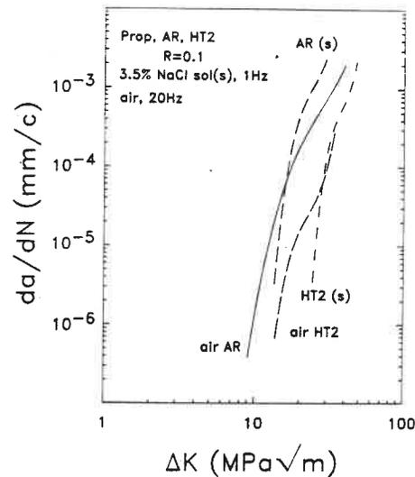
**Fig. 6.6:** Comparison of the crack growth curves in air and in the NaCl solution for the propeller specimens in the as-received and HT2 conditions.
