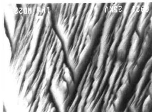
**Fig. 3.12:** Complex near-threshold facets for 316 s.s. tested in air. (a) stereographs pair (b) the matching aspect on the opposite fracture surface of the same region of (a).
