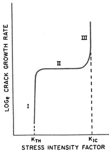
Fig. 1.12: Schematic diagram of typical three stages curve of crack propagation rate,  $\log da/dt$  vs. crack tip stress intensity,  $K$ , in SCC and HE cracking.
