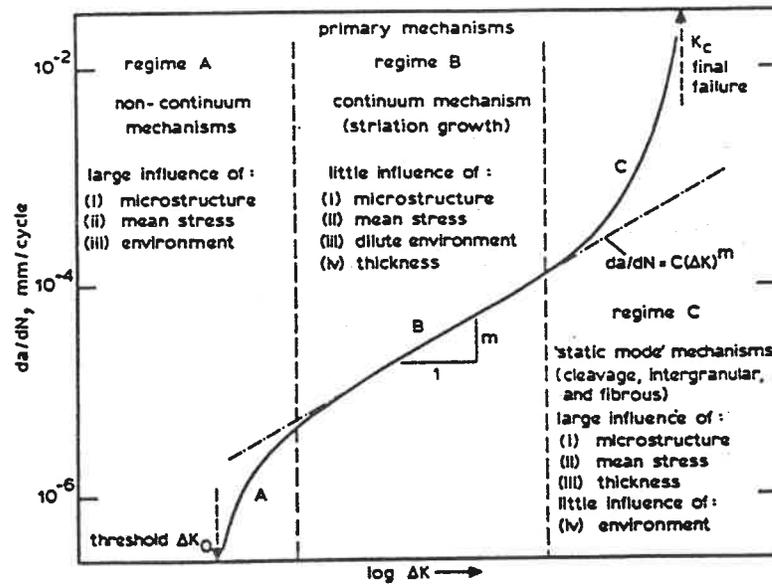
Fig. 1.1: Schematic variation of fatigue crack growth rate as function of stress intensity range (7).
