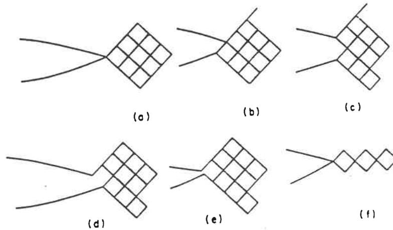
**Fig. 1.7:** Schematic of order of the localized slip which produces crystallographic striations (307).
