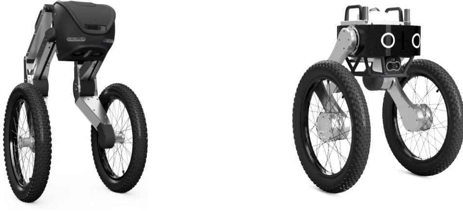
Figure 2.1 Ascento Robot evolution: The previous version (on the left) had a linkage system for each leg. The new version has pseudo-direct drive motors at the hips and knees, introducing additional degrees of freedom and allowing for more complex maneuvers.
