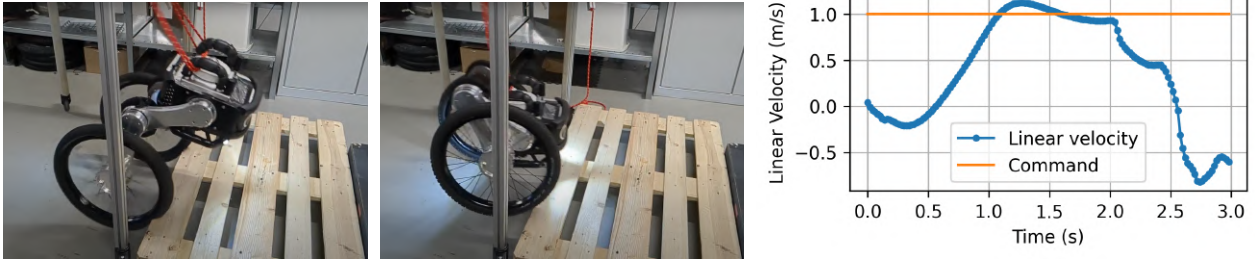
Figure 2.2 Stair climbing attempt with current velocity controller: Images of the Ascento robot attempting to climb a 15cm step with a constant velocity of 1m/s (left) and its corresponding linear velocity profile during the attempt (right).
