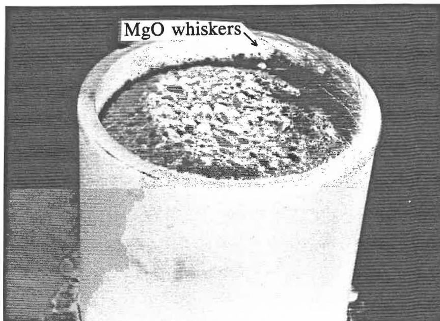
Figure 3.15 Observation of MgO whiskers formed on the hot face of brick sample with 15 wt% graphite (pre-oxidized in air at 1000°C for 5 h) after firing in CO at 1600°C for 5 h as a result of Mg vapour deposition.
