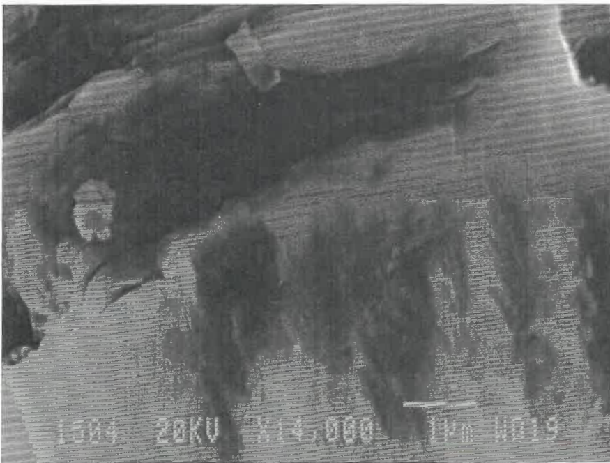
Figure 5.3b A transition from cleavage-like facet in an \alpha -phase grain to striation growth type near \alpha/\beta interface.
