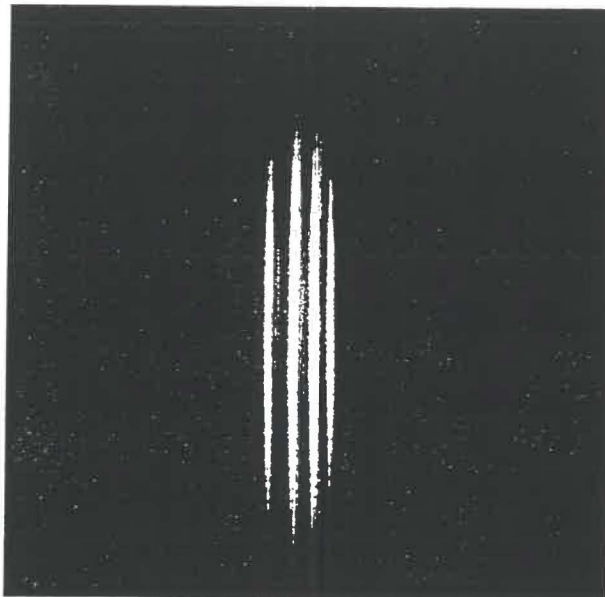
Fig. 2.6 Far-field patterns of m-lines coupled out by grating on a silver ion-exchanged channel waveguide. All guided modes are well excited.
