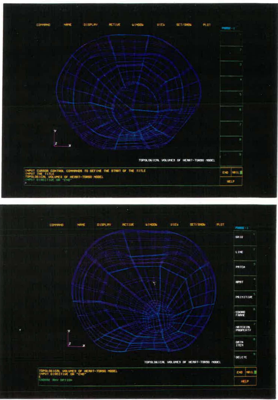
Figure 2.3: The topological volumes constructed from two consecutive cross-sectional images at (top) z = 24 and 25 , (bottom) z = 29 and 30 . The global coordinate system is shown in the lower left corner.
